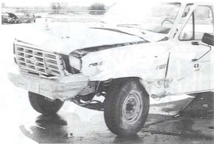
FIGURE 35. Vehicle Damage, Test NEOCR-5
