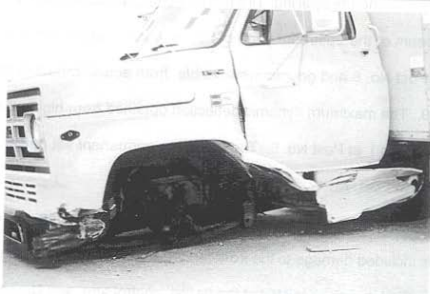
FIGURE 23. Test Vehicle Damage, Test NEOCR-3
