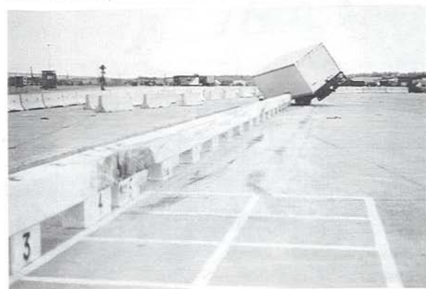
FIGURE 21. Bridge Rail Damage, Test NEOCR-3
