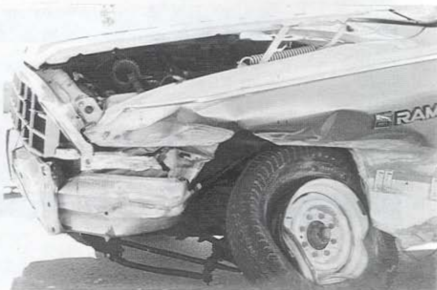
FIGURE 44. Vehicle Damage, Test NEOCR-6
