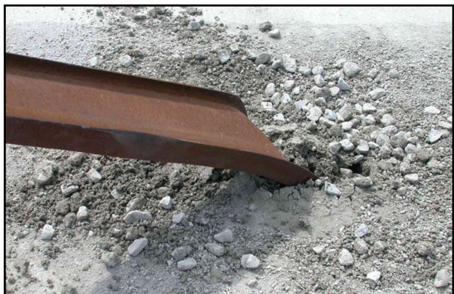
Figure 29. Post-Impact Image of CMPB-13, M203x9.7 (M8x6.5) Post in Soil
