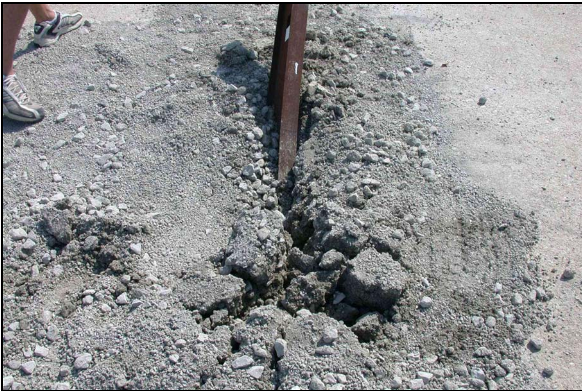
Figure 23. Post-Impact Image from CMPB-7, M203x9.7 (M8x6.5) Post in Soil
