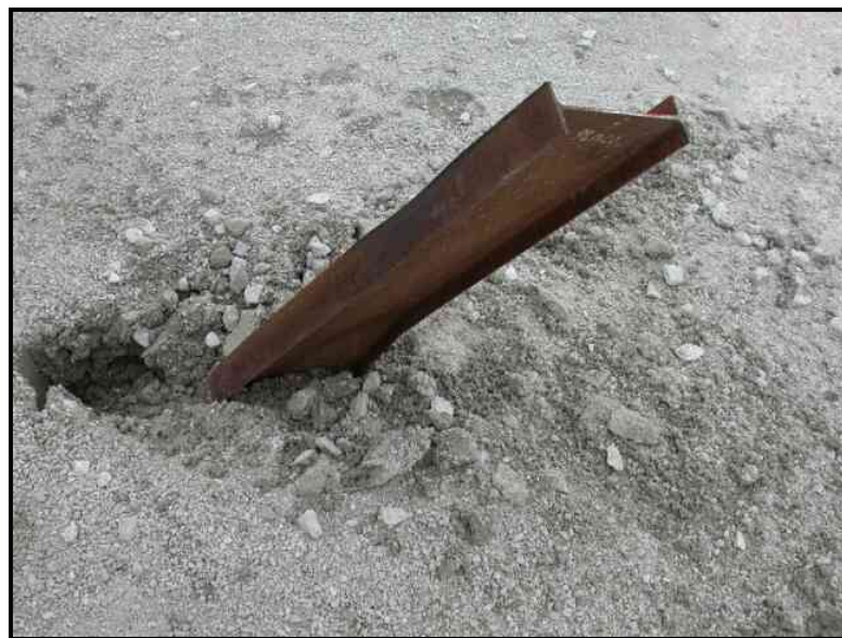
Figure 26. Post-Impact Image of CMPB-10, M203x9.7 (M8x6.5) Post in Soil
