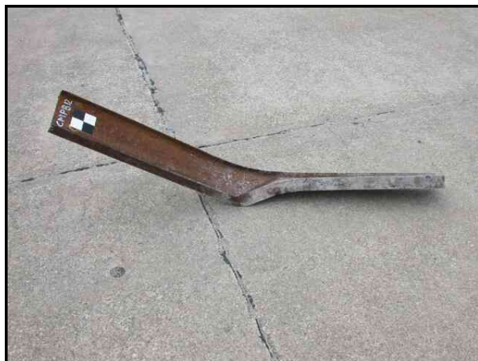
Figure 28. Post-Impact Image of CMPB-11, M203x9.7 (M8x6.5) Post in Soil
