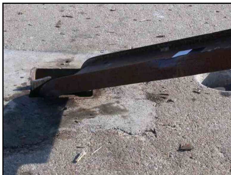
Figure 19. Post-Impact Image of CMPB-3, M203x9.7 (M8x6.5) Post in Concrete
