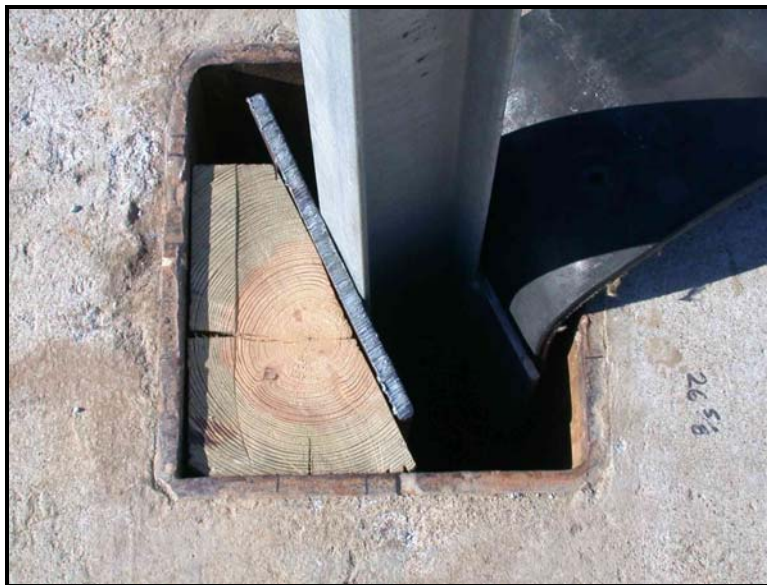
Figure 5. Typical Post and Wood Block Setup for Tests CMPB-1 through CMPB-6
