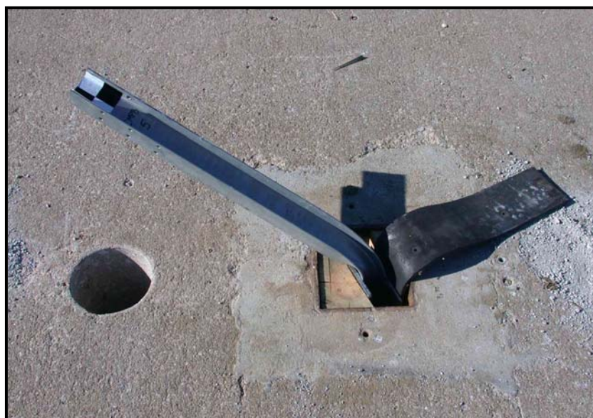
Figure 21. Post-Impact Image of CMPB-5, S76x8.5 (S3x5.7) Post in Concrete
