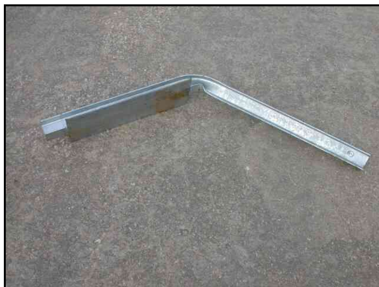
Figure 22. Post-Impact Image of CMPB-6, S76x8.5 (S3x5.7) Post in Concrete
