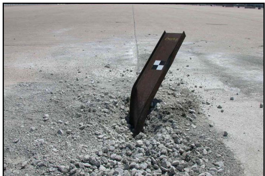
Figure 24. Post-Impact Image of CMPB-8, M203x9.7 (M8x6.5) Post in Soil
