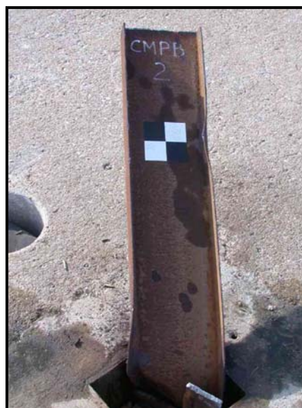
Figure 18. Post-Impact Image of CMPB-2, M203x9.7 (M8x6.5) Post in Concrete
