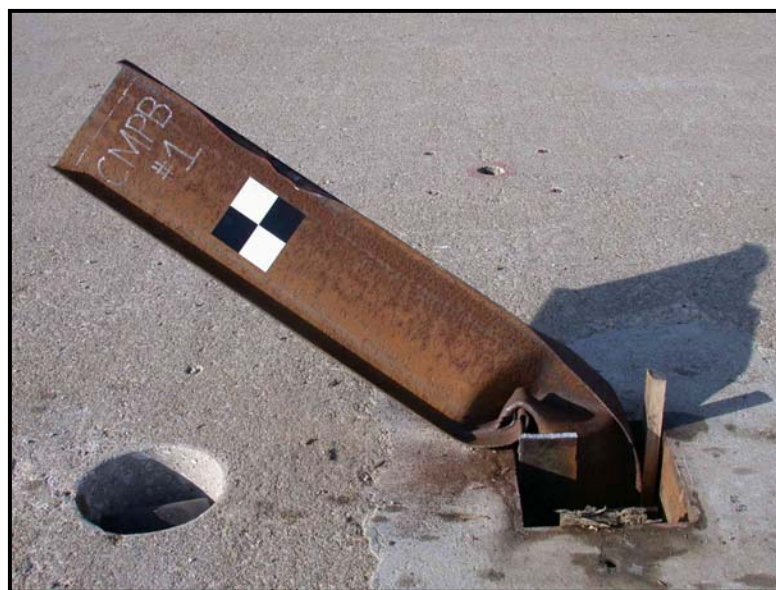
Figure 17. Post-Impact Image of CMPB-1, M203x9.7 (M8x6.5) Post in Concrete
