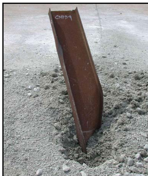
Figure 25. Post-Impact Image of CMPB-9, M203x9.7 (M8x6.5) Post in Soil
