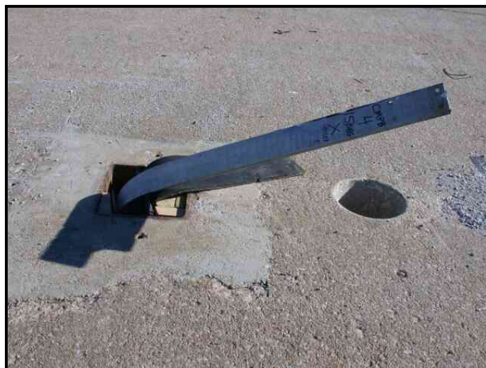
Figure 20. Post-Impact Image of CMPB-4, S76x8.5 (S3x5.7) Post in Concrete
