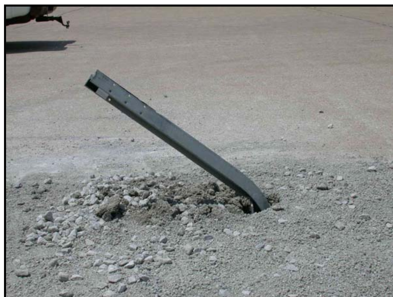
Figure 30. Post-Impact Image of CMPB-14, S76x8.5 (S3x5.7) Post in Soil
