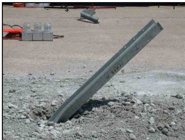
Figure 31. Post-Impact Image of CMPB-15, S76x8.5 (S3x5.7) Post in Soil
