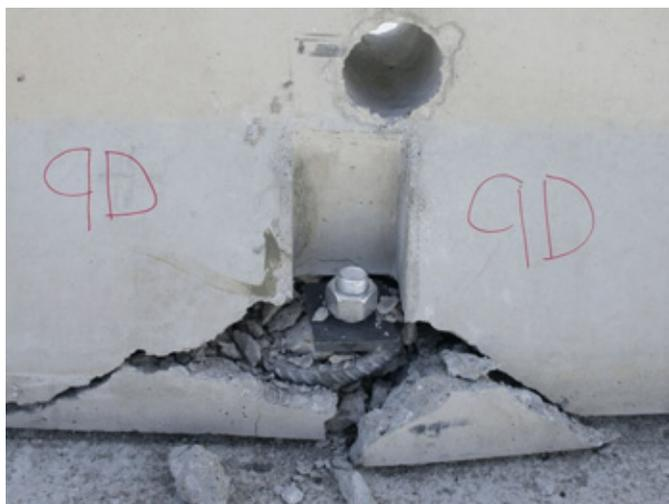
Figure 29. Barrier No. 9 Tie-Down Anchor Damage, Test KTB-1
