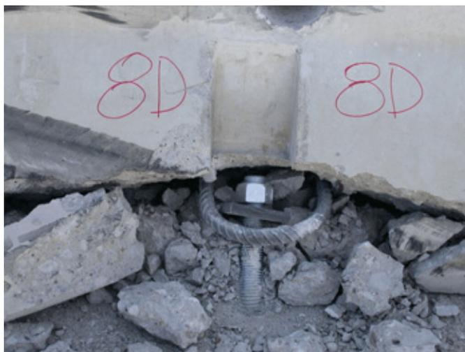
Figure 28. Barrier No. 8 Tie-Down Anchor Damage, Test KTB-1
