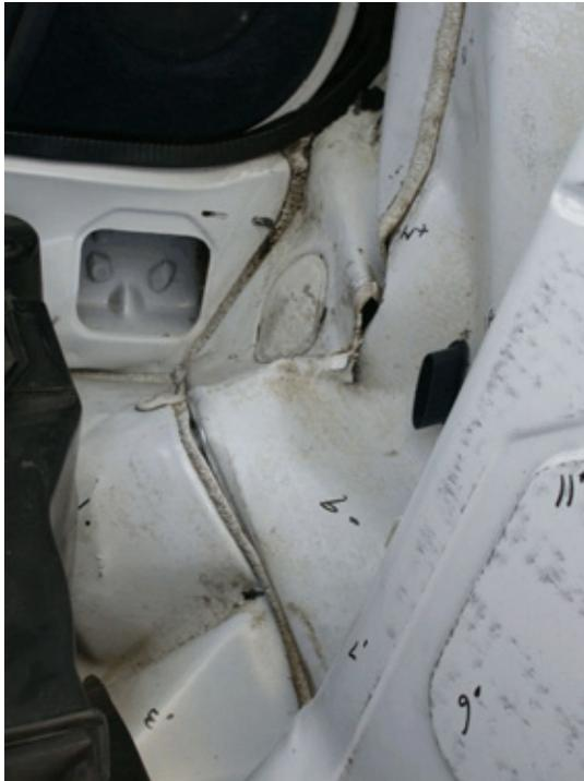
Figure 34. Occupant Compartment Damage, Test KTB-1
