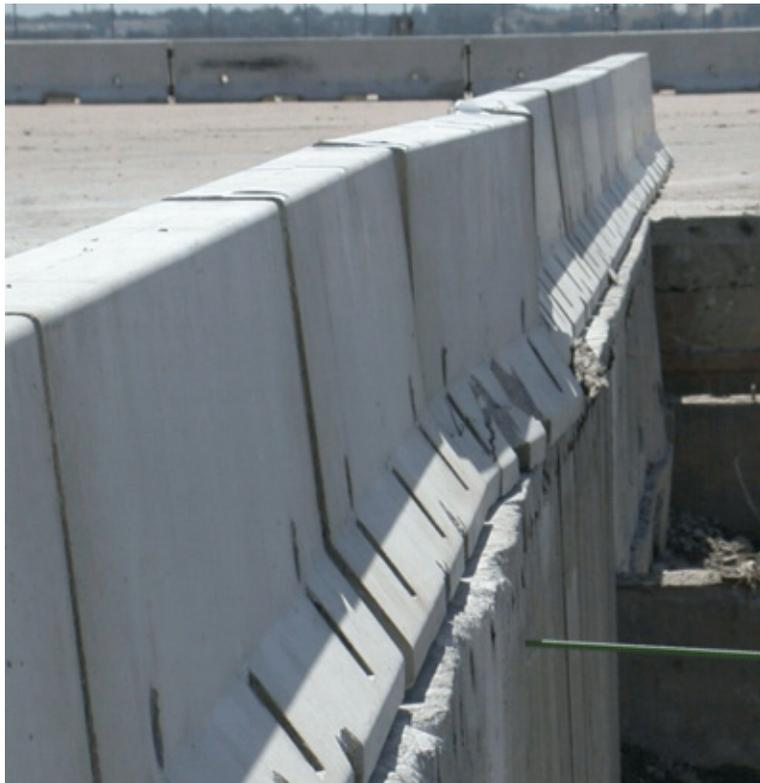
Figure 25. System Damage, Test KTB-1
