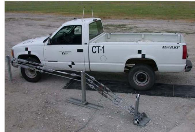
Figure 93. CT-1 Length-of-Need Test Setup and Impact Location
