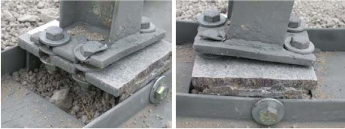
Figure 96. CT-1 Slip Base Damage
