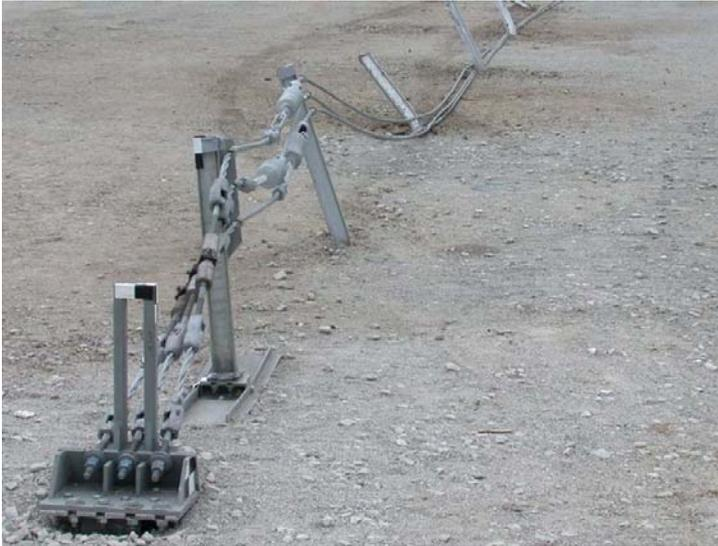
Figure 94. Aftermath of CT-1 Length-of-Need Crash Test
