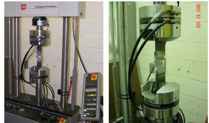
Figure 62. MTS Machine with Slip Base Jig
