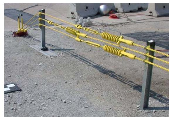
Figure 6. MwRSF Cable Guardrail System End Terminal, CT-2 Crash Test
