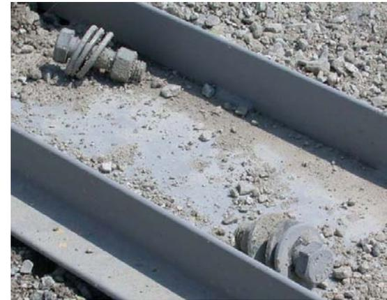
Figure 52. Bolt, Nut, and Washers Following Slip Base Activation (CT-2)
