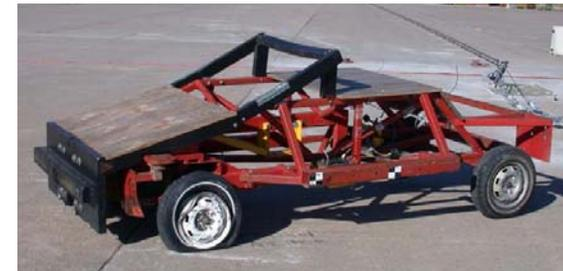
Figure 85. CTB-4, Prototype End Terminal and Bogie Vehicle
