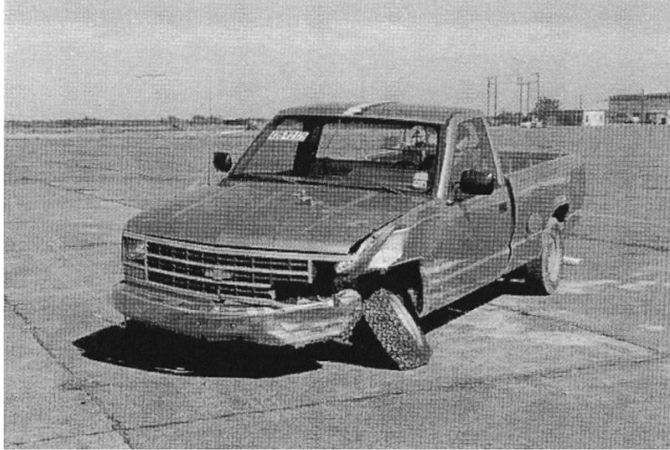
**Figure 23. Vehicle Damage After Test No. 405421-1 [14]**
