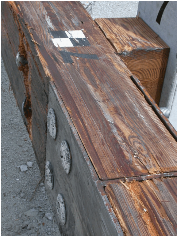
Figure 36. System Damage Between Post Nos. 6 and 7, Test MNTR-1
