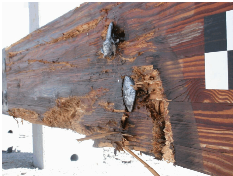
Figure 35. System Damage at Post No. 6, Test MNTR-1
