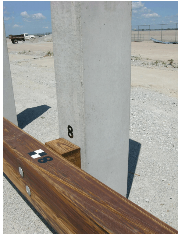
Figure 38. Post Damage and Movement at Post Nos. 6 through 8, Test MNTR-1
