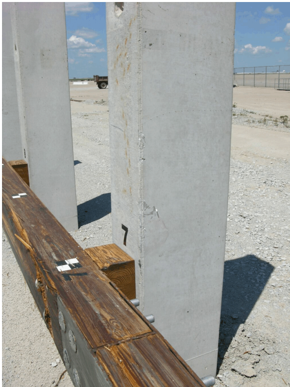
Figure 38. Post Damage and Movement at Post Nos. 6 through 8, Test MNTR-1
