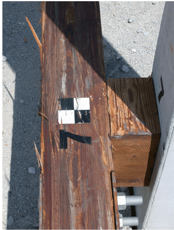
Figure 36. System Damage Between Post Nos. 6 and 7, Test MNTR-1
