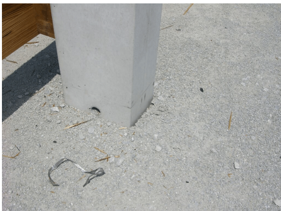
Figure 39. Soil Failure at Post Nos. 6 through 8, Test MNTR-1
