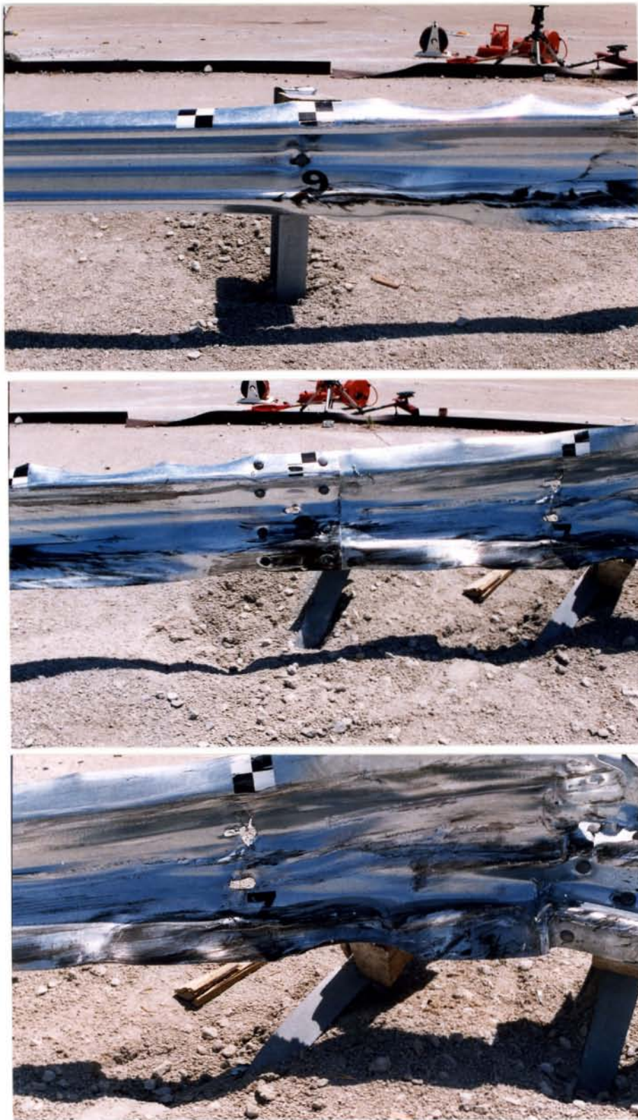
Figure 45. W-beam to Thrie Beam Transition Damage, Test MWT-2
