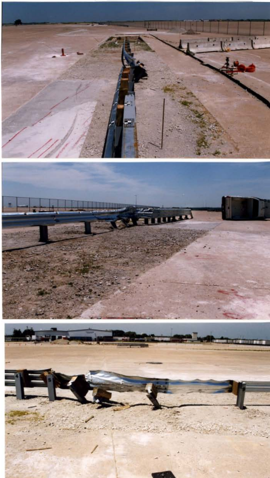
Figure 44. W-beam to Thrie Beam Transition Damage, Test MWT-2
