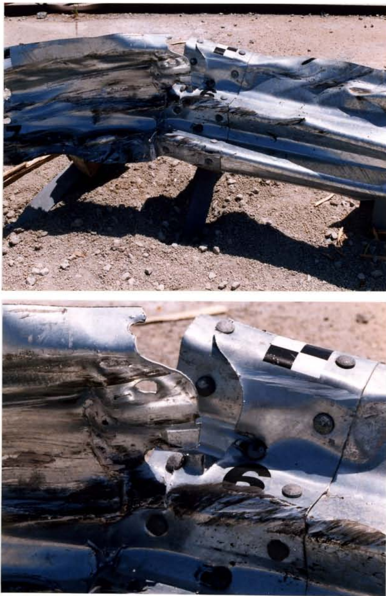
Figure 46. W-beam to Thrie Beam Transition Damage, Test MWT-2
