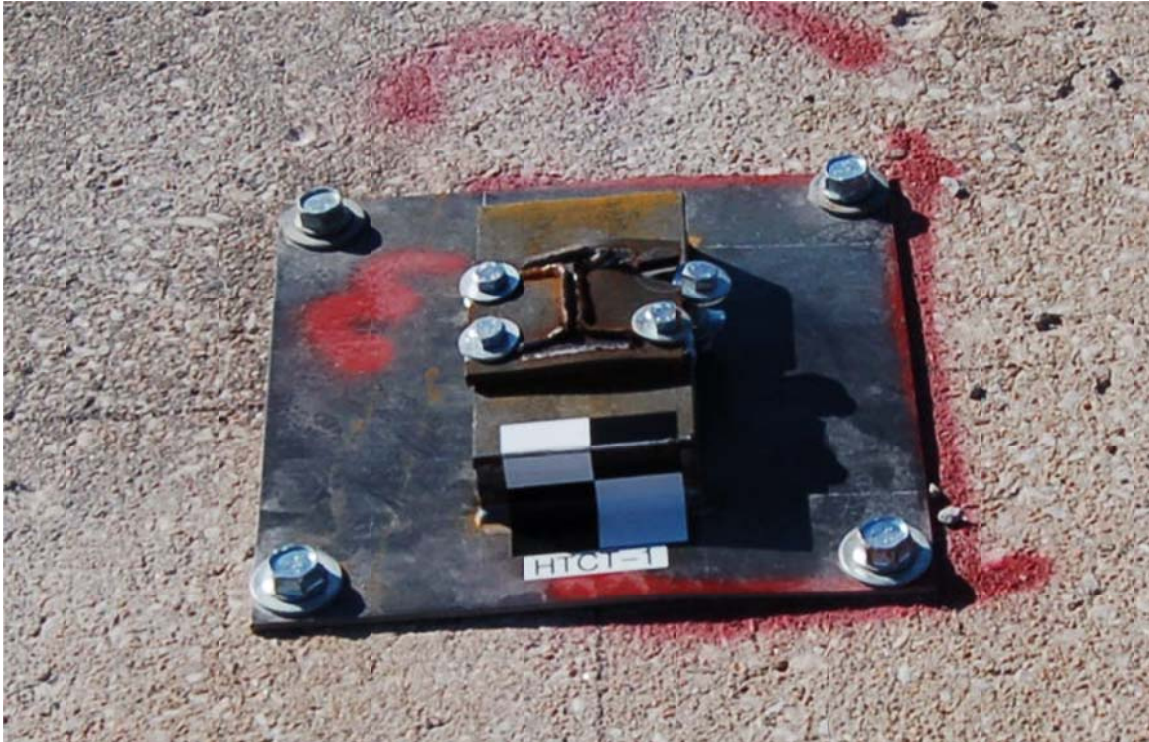
Downstream Slip Base Post Assembly
