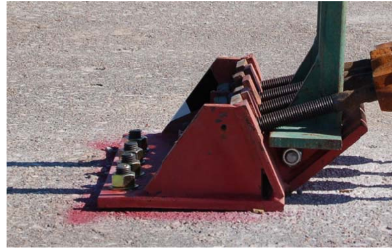
Upstream Cable Anchor Bracket Assembly – Pre-Test
