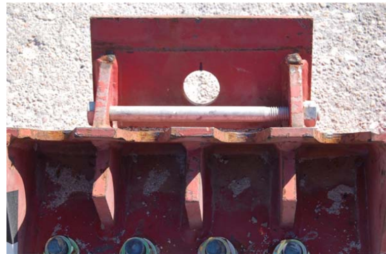
Upstream Cable Anchor Bracket Assembly – Post-Test
