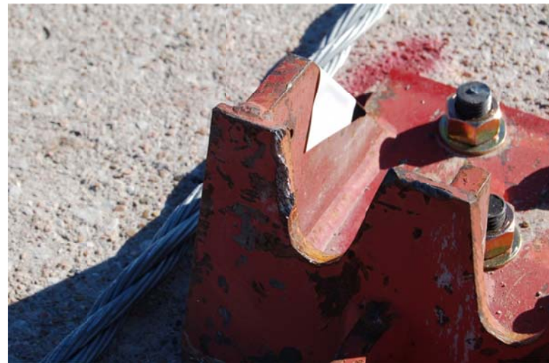
Downstream Cable Anchor Bracket Assembly – Post-Test
