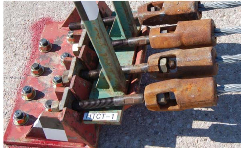
Downstream Cable Anchor Bracket Assembly – Pre-Test
