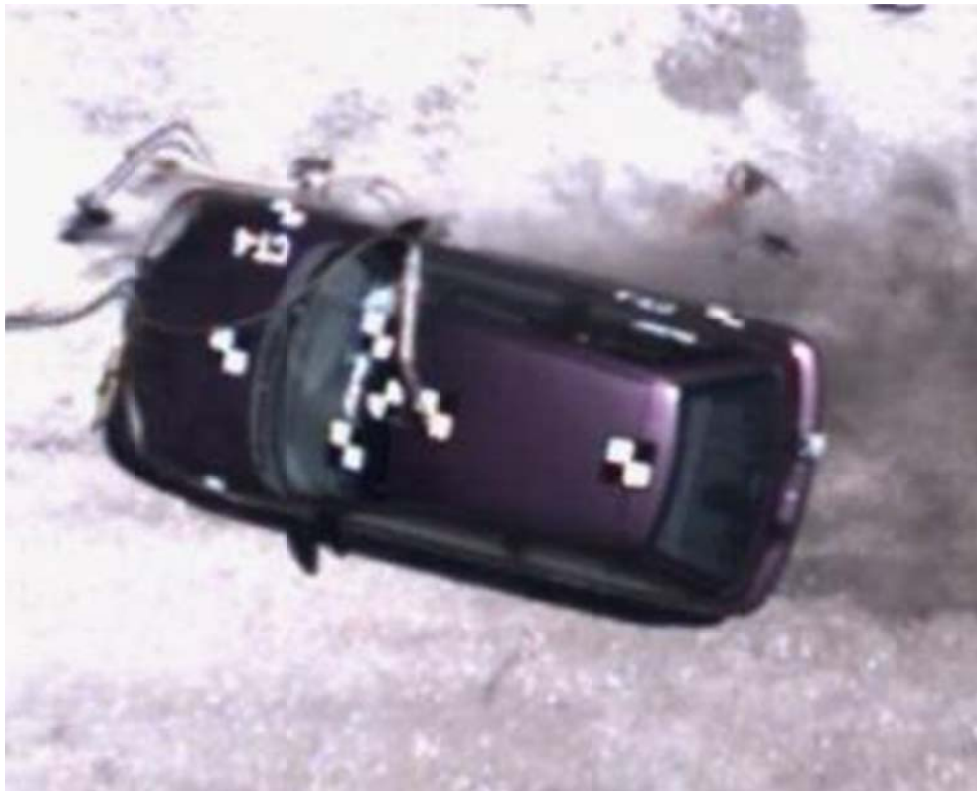
Figure 23. Geo Metro Overriding System Debris
