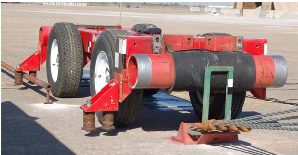
Figure 49. Rigid Frame Bogie on Guidance Track
