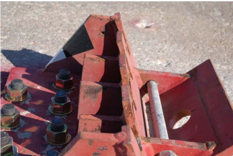
Upstream Cable Anchor Bracket Assembly – Post-Test
