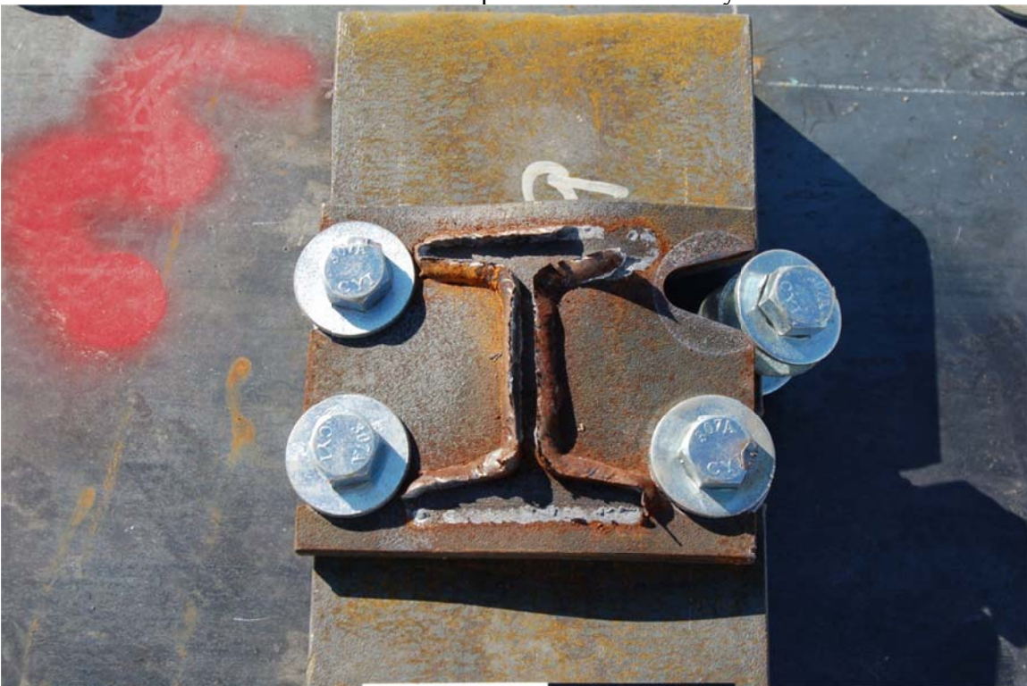
Downstream Slip Base Post Assembly
