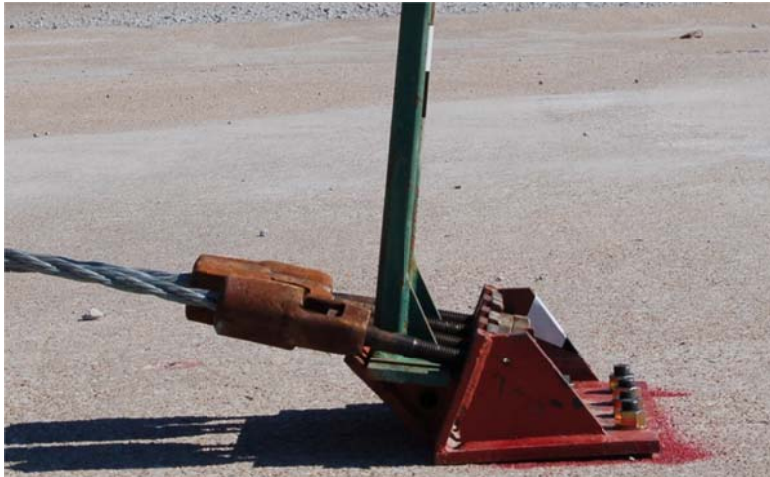
Downstream Cable Anchor Bracket Assembly – Pre-Test
