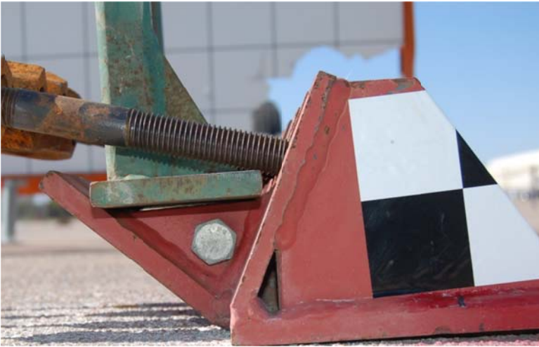
Upstream Cable Anchor Bracket Assembly – Pre-Test
