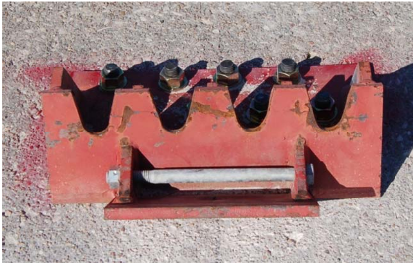
Figure 65. Upstream Cable Anchor Damage Comparison, Test No. HTCT-1 vs. Simulation
