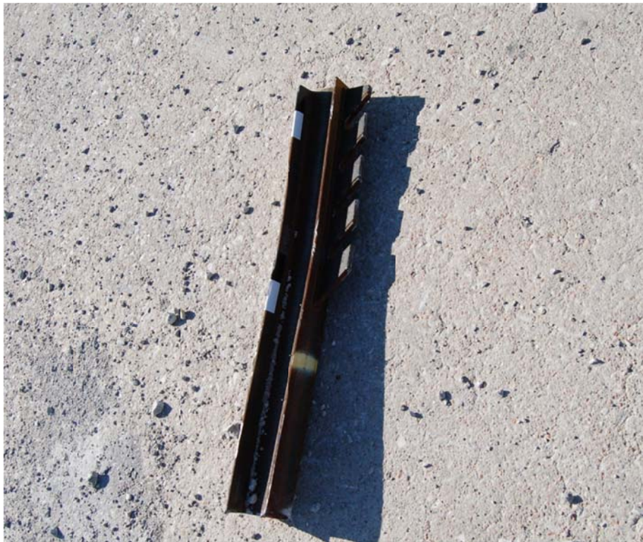
Downstream Slip Base Post Assembly
