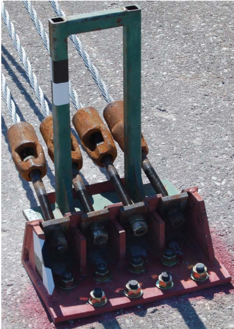
Figure 34. Cable Anchor Bracket and Finite Element Model
