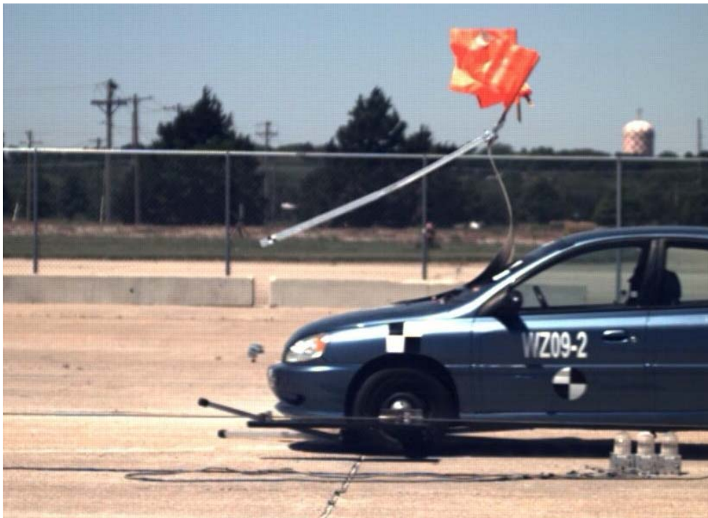
Figure 103. System No. 3A, Frangible Mast
