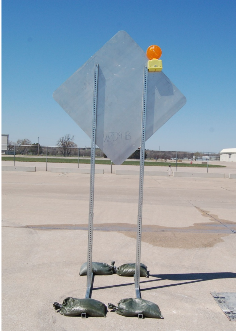
Figure 16. System No. 1B Details, Test No. WZ09-1
