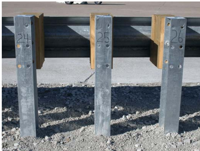
Figure 122. Reduced Post Spacing Midwest Guardrail System
