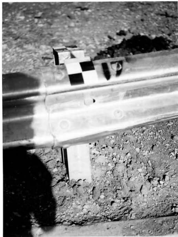
Figure 23. Barrier and Post Permanent Deformation Near Post Nos. 16 and 17
