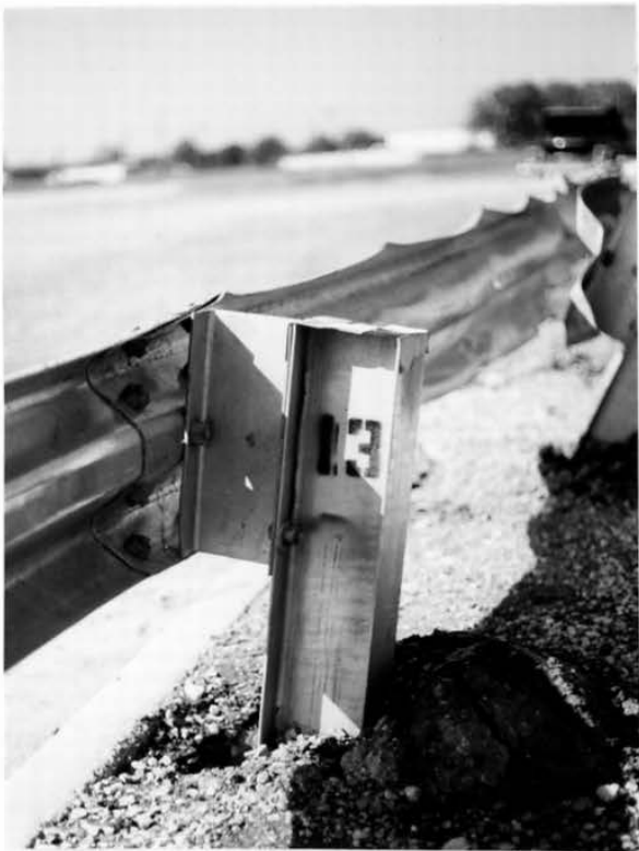
Figure 21. Barrier and Post Permanent Deformation Near Post Nos. 12 and 13
