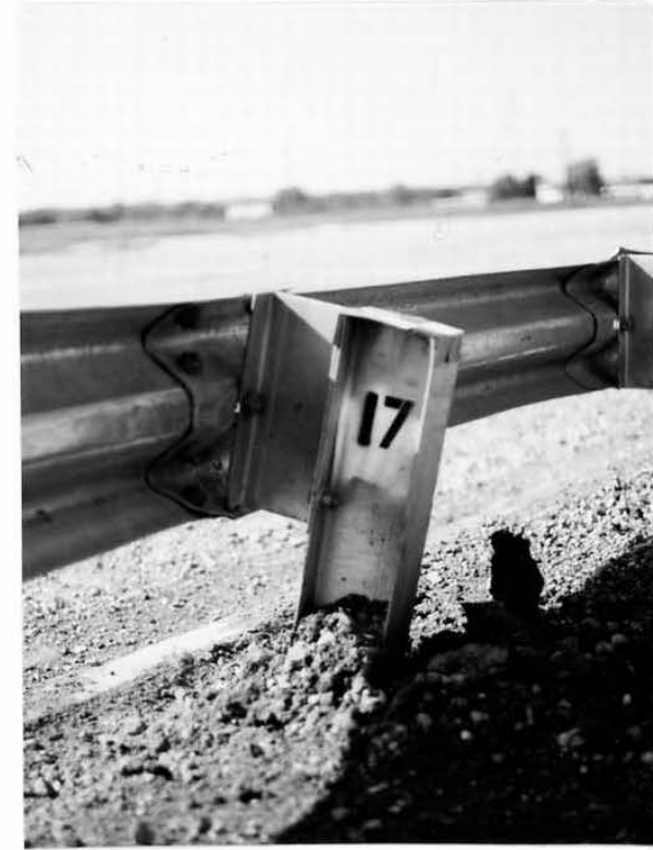
Figure 23. Barrier and Post Permanent Deformation Near Post Nos. 16 and 17
