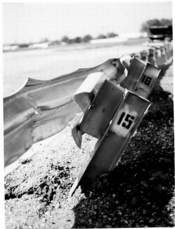
Figure 22. Barrier and Post Permanent Deformation Near Post Nos. 14 and 15
