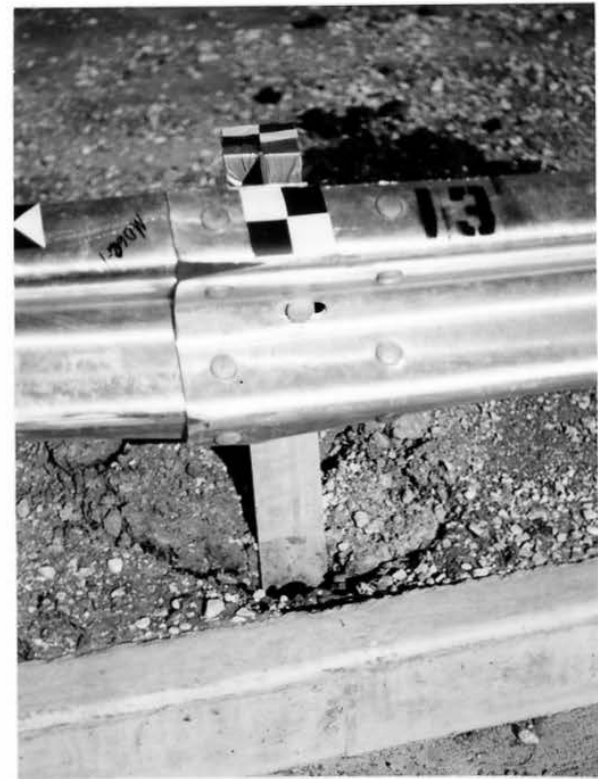
Figure 21. Barrier and Post Permanent Deformation Near Post Nos. 12 and 13
