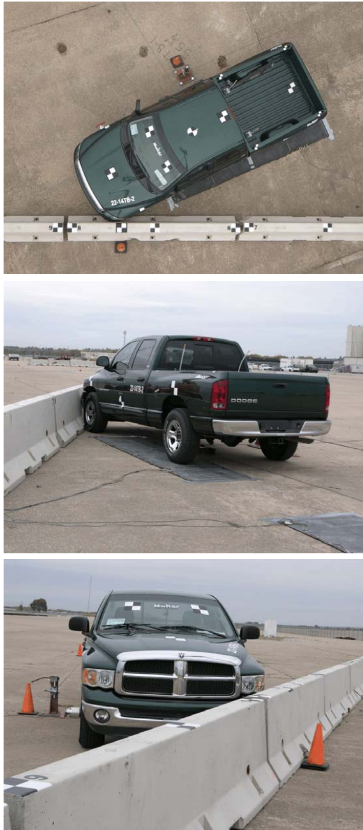
Figure 20. Impact Location, Test 2214TB-2
