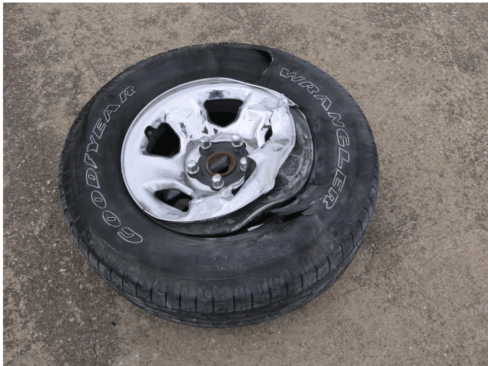
Figure 28. Vehicle Damage, Test 2214TB-2
