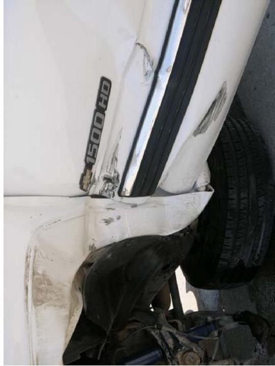
Figure 38. Vehicle Damage, Test 2214T-1
