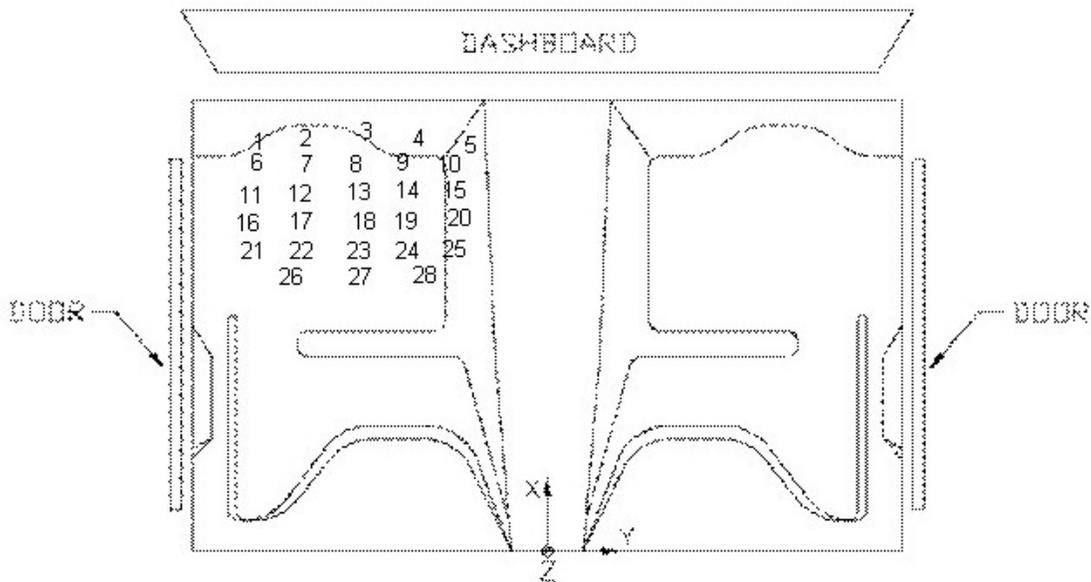
Figure C-2. Occupant Compartment Deformation Data - Set 2, Test 2214T-1
