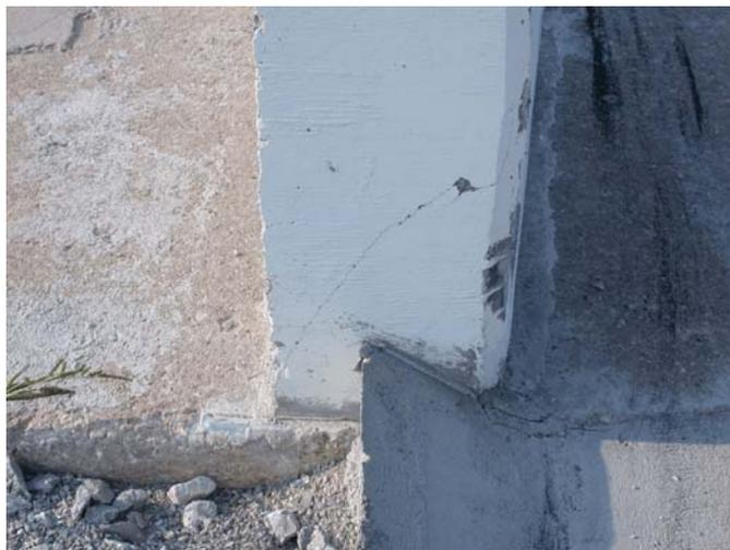
Figure 35. Concrete Barrier System Damage, Test 2214T-1
