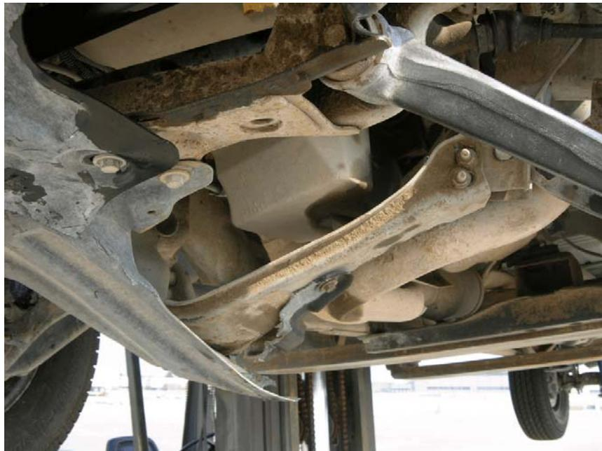
Figure 40. Vehicle Undercarriage Damage, Test 2214T-1
