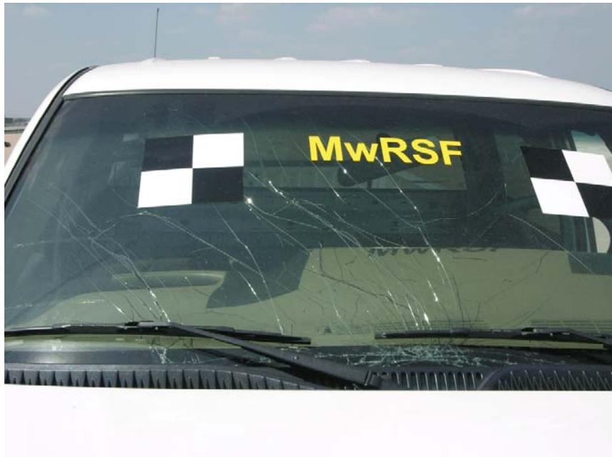
Figure 39. Vehicle Windshield Damage, Test 2214T-1
