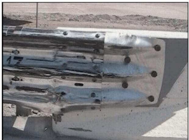
Figure 34. Approach Guardrail Transition System Damage, Test 2214T-1
