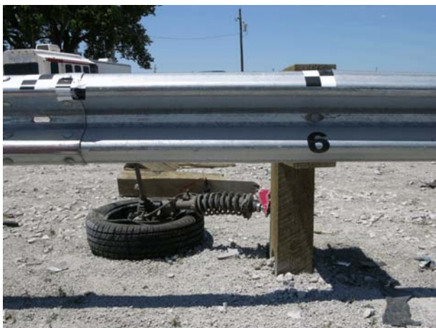
Figure 33. Midwest Guardrail System End Terminal Damage, Test 2214TT-1
