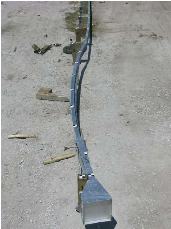
Figure 32. Midwest Guardrail System End Terminal Damage, Test 2214TT-1
