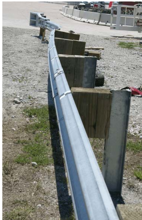
Figure 32. Midwest Guardrail System End Terminal Damage, Test 2214TT-1
