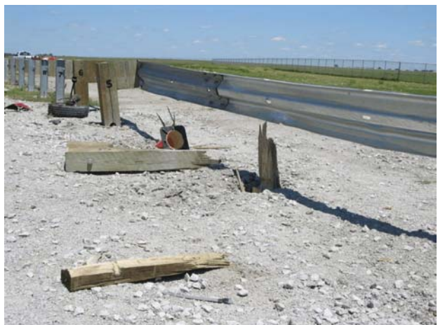
Figure 33. Midwest Guardrail System End Terminal Damage, Test 2214TT-1
