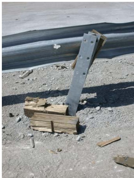
Figure 27. Post Nos. 16 through 20 Damage, Test 2214WB-1
