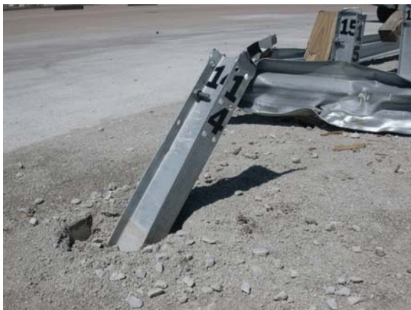
Figure 26. Post Nos. 10 through 15 Damage, Test 2214WB-1
