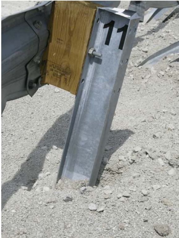
Figure 25. Post Nos. 9 through 12 Damage, Test 2214WB-2
