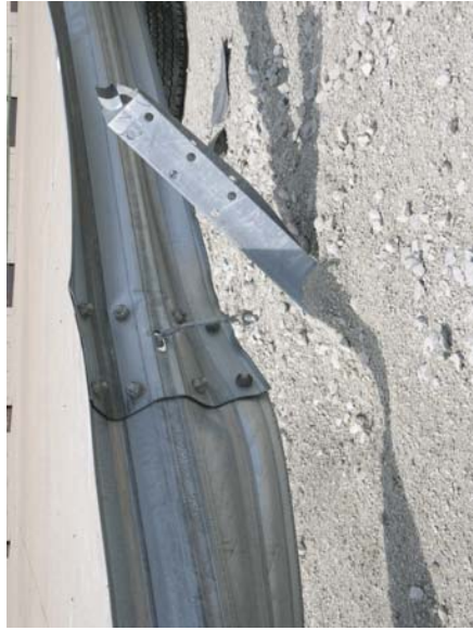
Figure 26. Post Nos. 13 through 16 Damage, Test 2214WB-2
