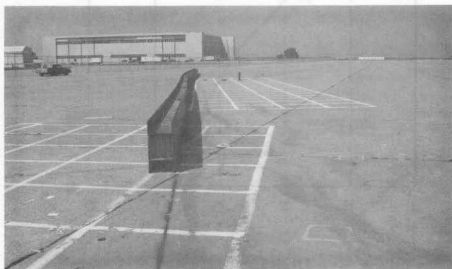
FIGURE 14. PHOTOGRAPHS OF BARRIER RAIL AFTER IMPACT.
