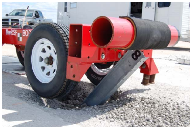
Figure 1. Impacted Post Contacting Backslope of Testing Pit
