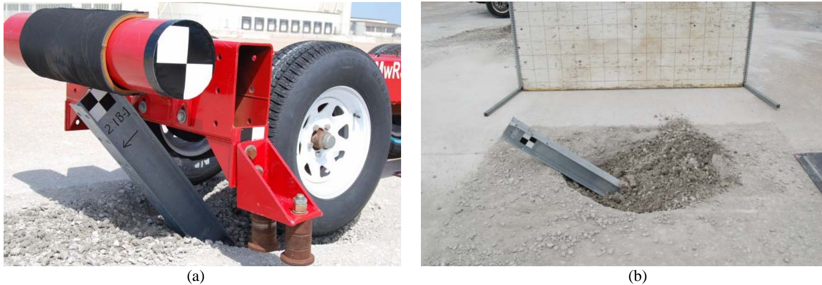
Figure 10. Post-Impact Image of (a) MGS2-1B1 and (b) MGS2-1B10
