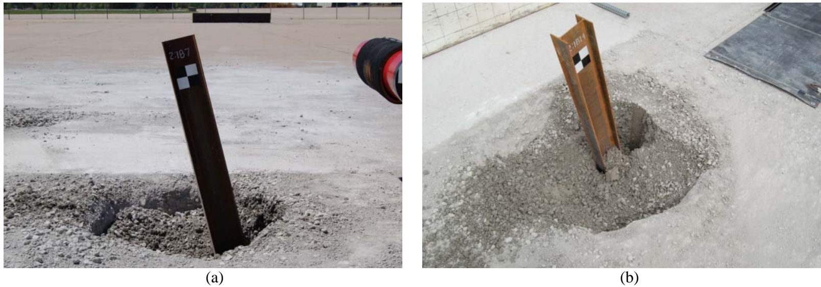
Figure 28. Post-Impact Image of (a) MGS2-1B7 and (b) MGS2-1B14
