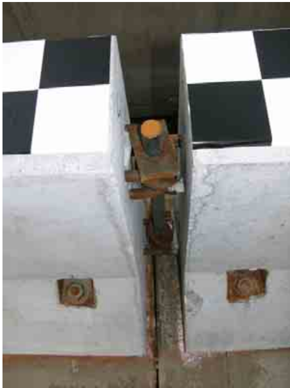
Figure 37. Barrier Connection Deformations Between Barrier Nos. 8 and 9, Test KSC-1
