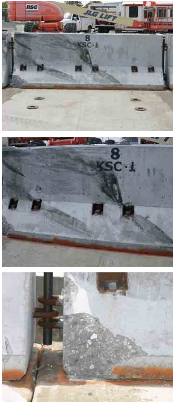
Figure 36. Barrier No. 8 Damage, Test KSC-1
