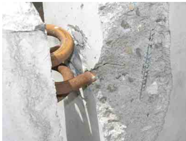
Figure 38. Barrier Connection Damage Between Barrier Nos. 6 and 7, Test KSC-1 (pin removed)
