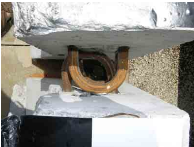
Figure 38. Barrier Connection Damage Between Barrier Nos. 6 and 7, Test KSC-1 (pin removed)
