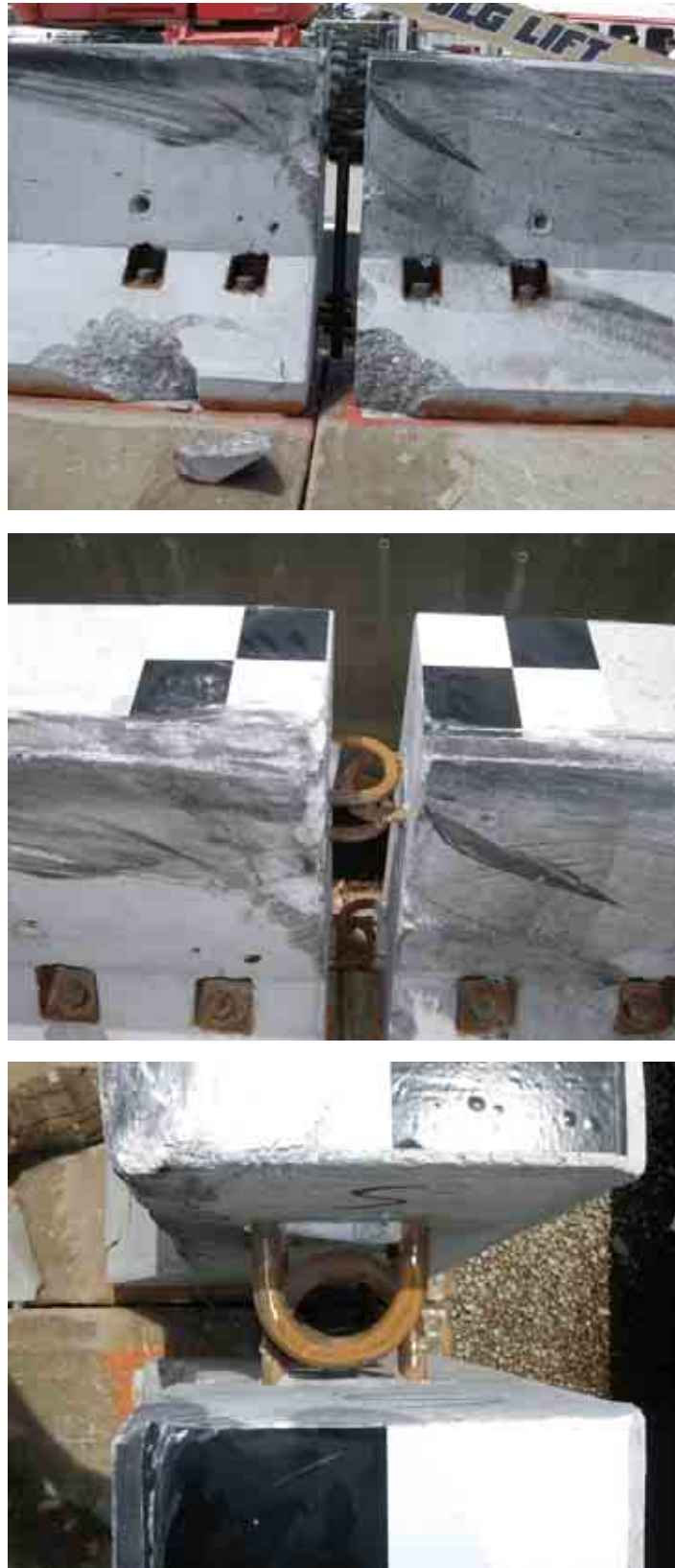
Figure 39. Barrier Connection Damage Between Barrier Nos. 7 and 8, Test KSC-1 (pin removed)
