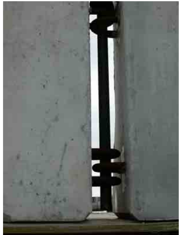
Figure 37. Barrier Connection Deformations Between Barrier Nos. 8 and 9, Test KSC-1
