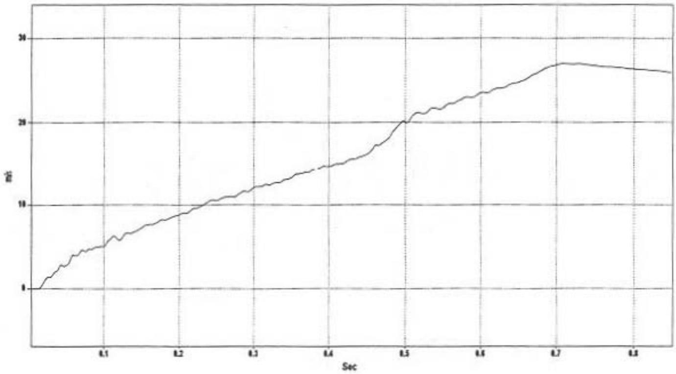
Figure C-20. Longitudinal Change in Velocity, Test BEST-9.
