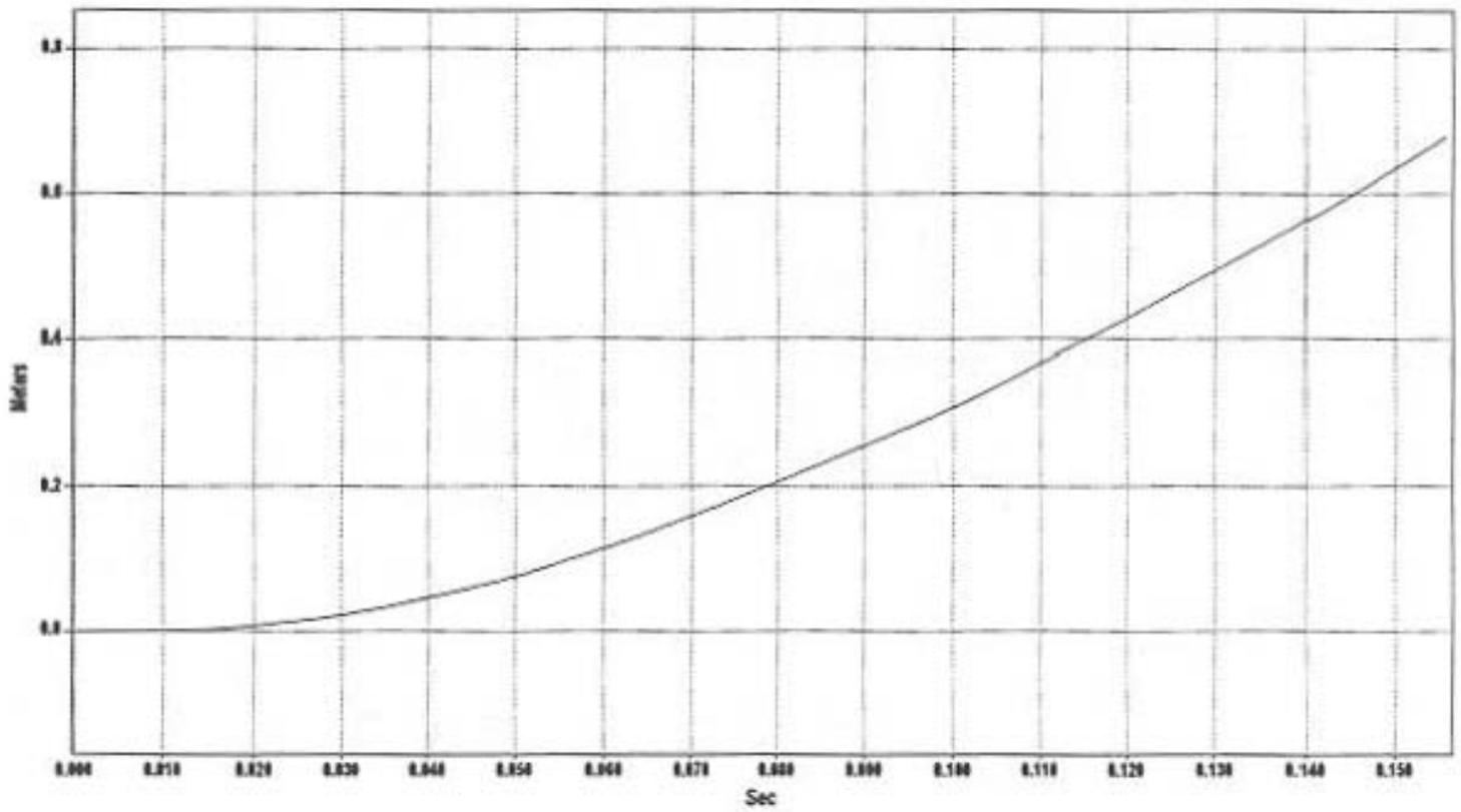
Figure C-21. Relative Longitudinal Occupant Displacement, Test BEST-9.
