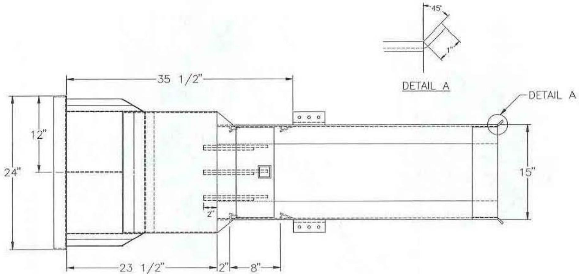
Figure 4. Side View of the BEST Impact Head for Tests BEST-2,3, and 4.
