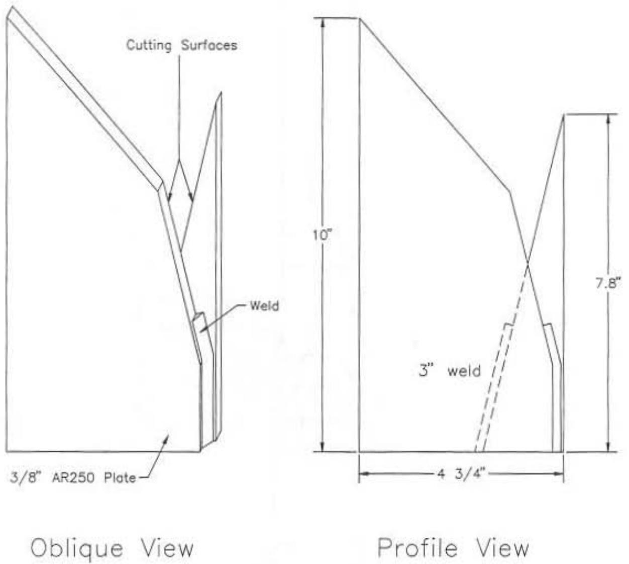
Figure 8. Details of BEST Cutting Teeth.
