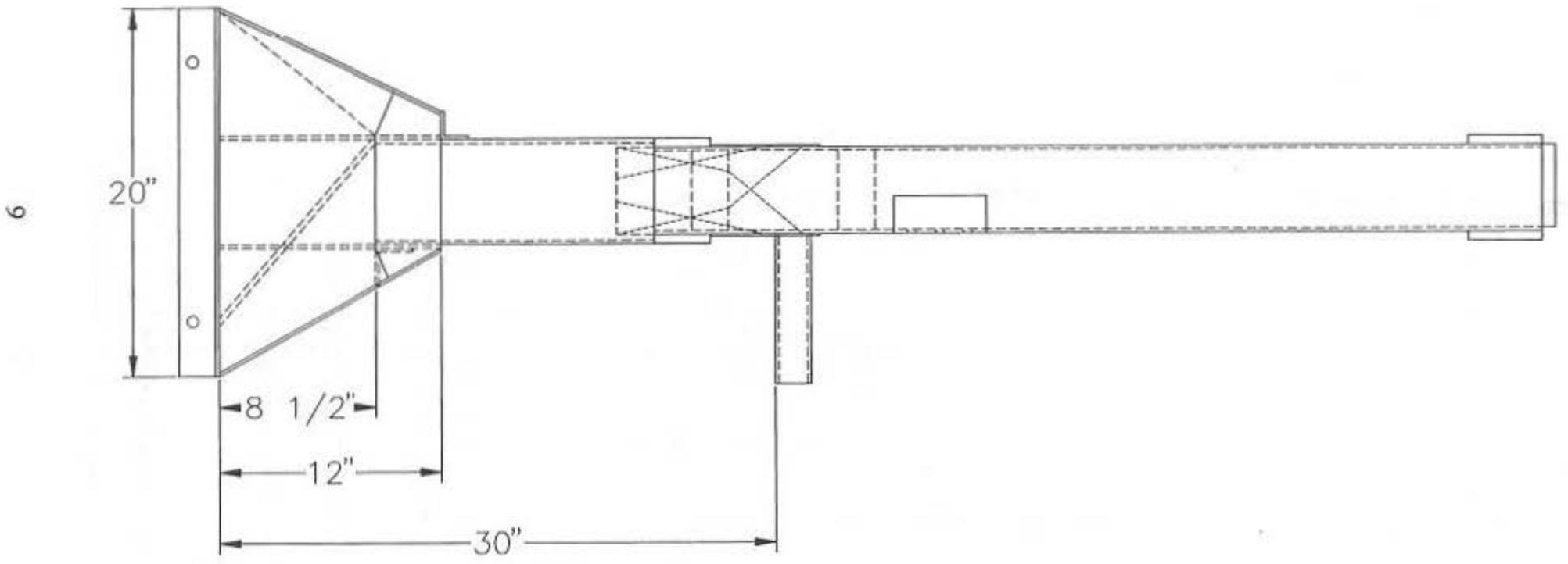
Figure 5. Top View of BEST Impact Head for Tests BEST-2,3, and 4.
