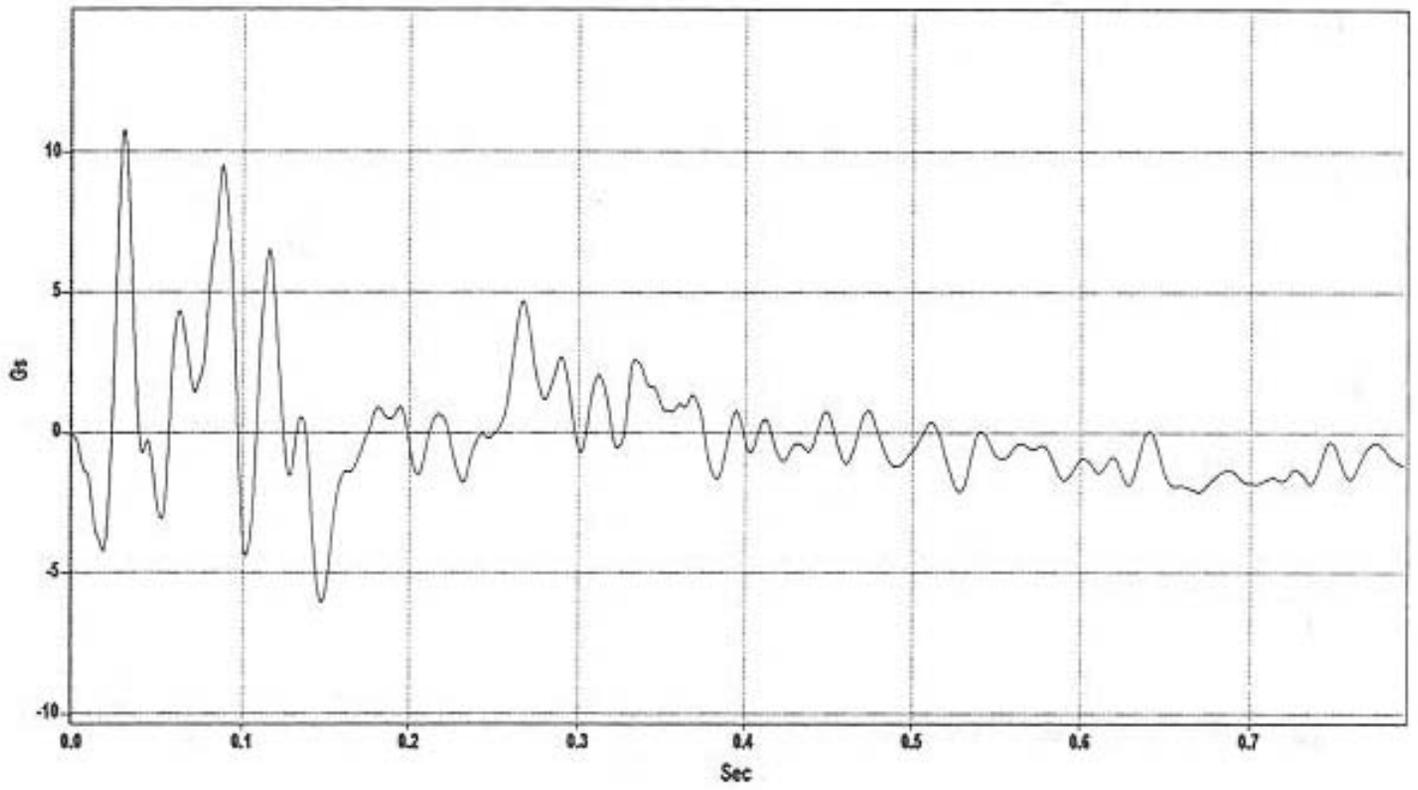
Figure C-10. Lateral Deceleration, Test BEST-4.
