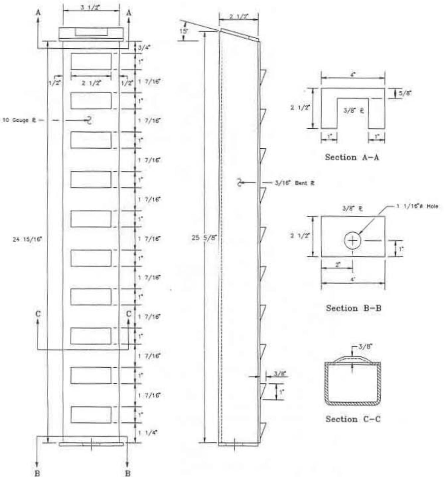
Figure 11. Breakaway Cable Anchor Box Details.
