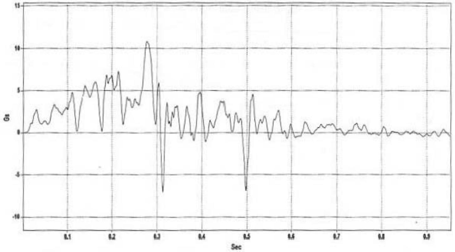
Figure C-1. Longitudinal Deceleration, Test BEST-3.
