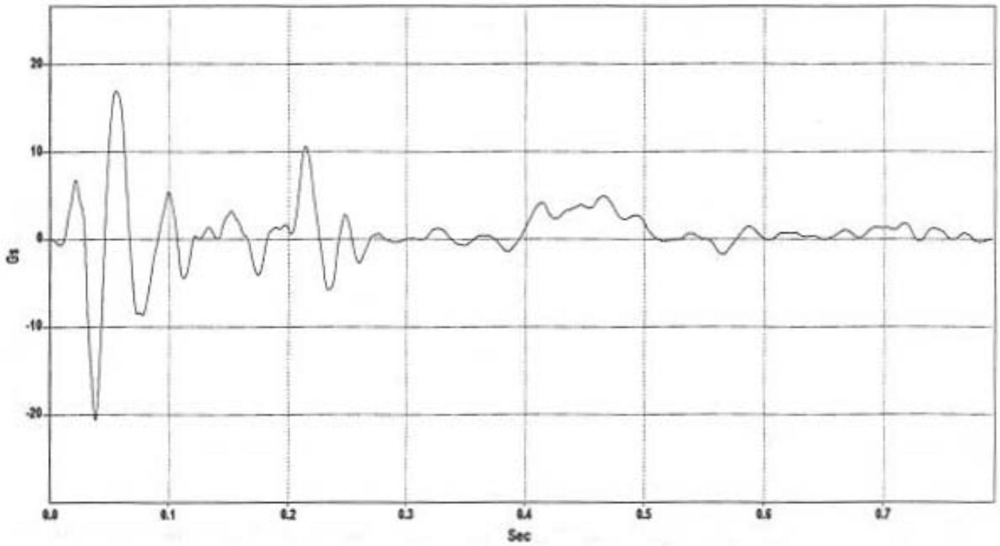
Figure C-16. Lateral Deceleration, Test BEST-8.
