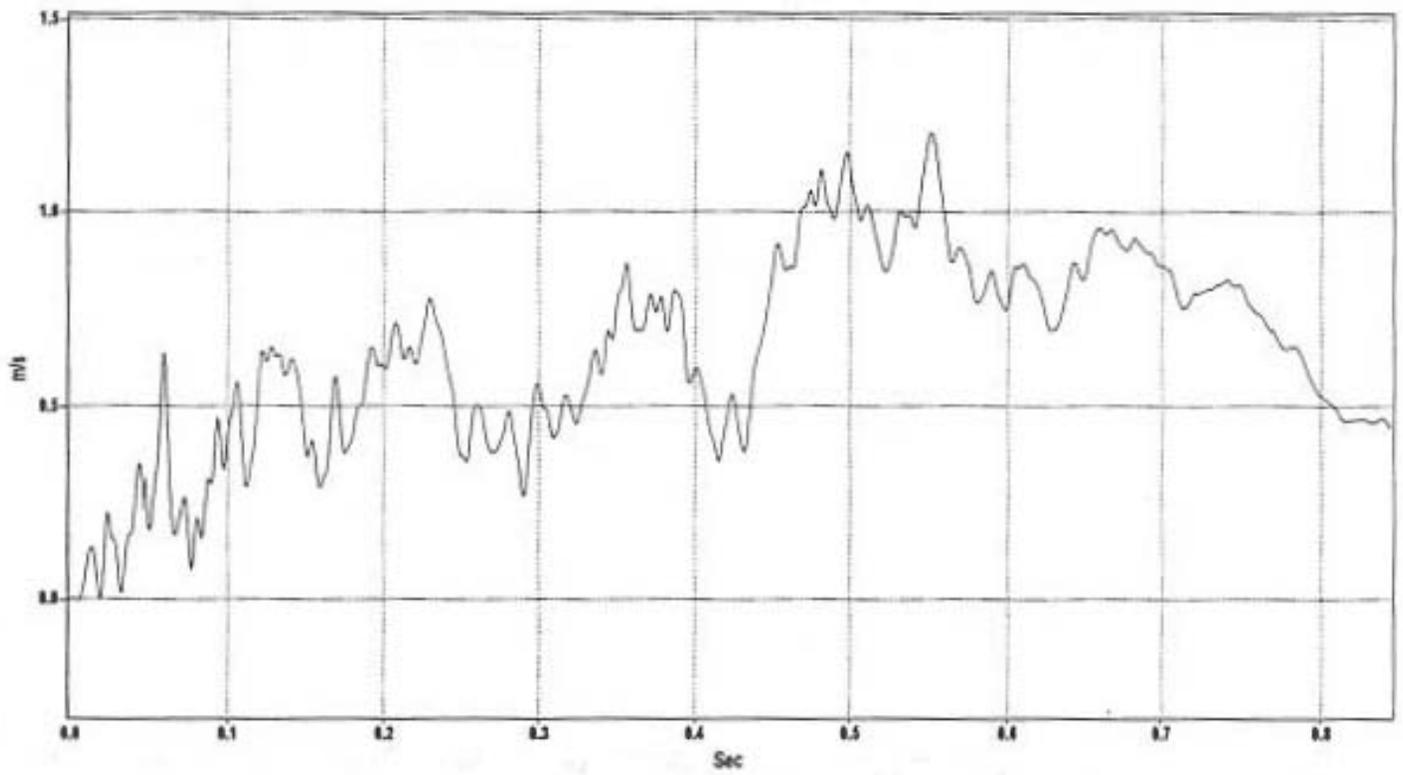
Figure C-23. Lateral Change in Velocity, Test BEST-9.
