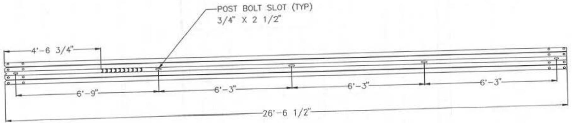
Figure 13. Terminal W-beam Details.
