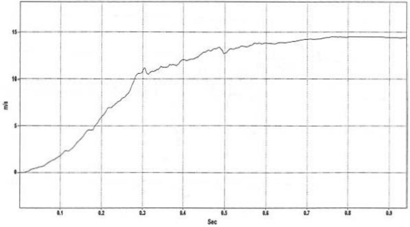
Figure C-2. Longitudinal Change in Velocity, Test BEST-3.
