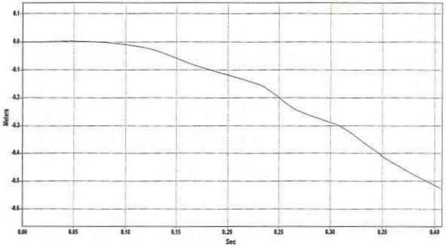
Figure C-30. Relative Lateral Occupant Displacement, Test BEST-10.
