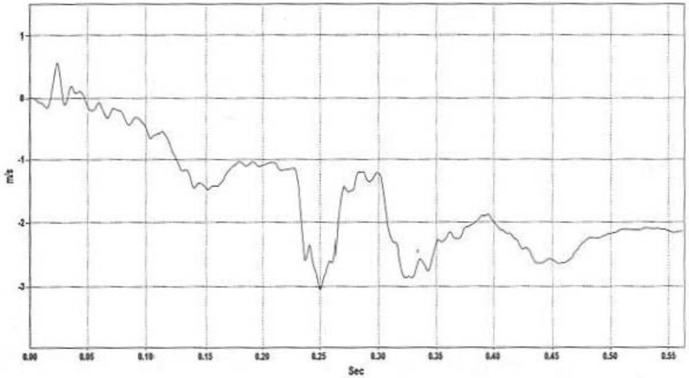
Figure C-29. Lateral Change in Velocity, Test BEST-10.
