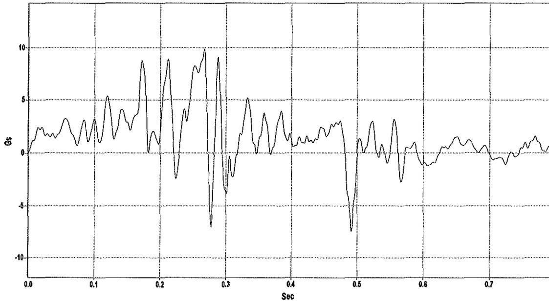
Figure C-4. Lateral Deceleration, Test BEST-3.
