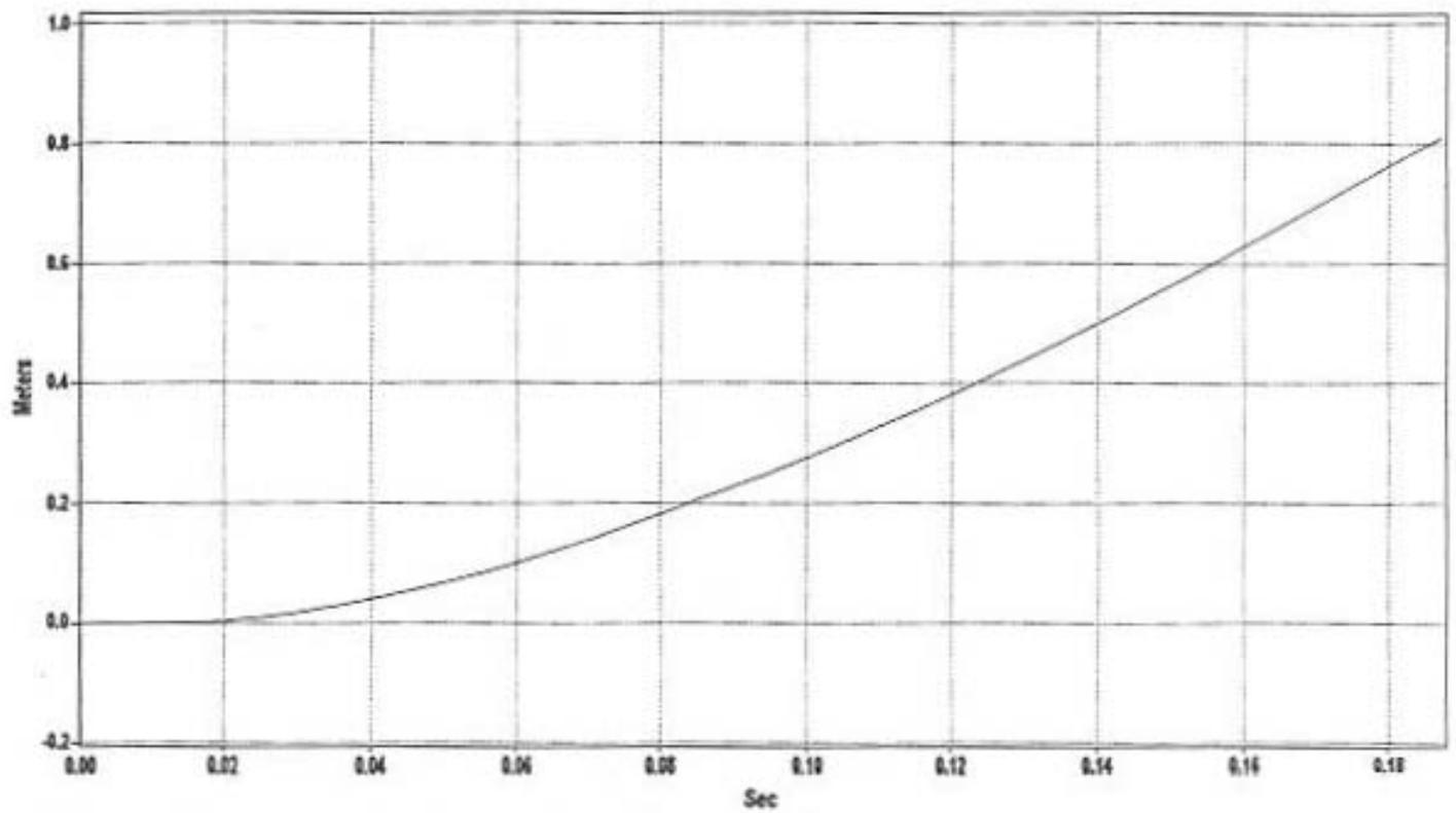
Figure C-27. Relative Longitudinal Occupant Displacement, Test BEST-10.
