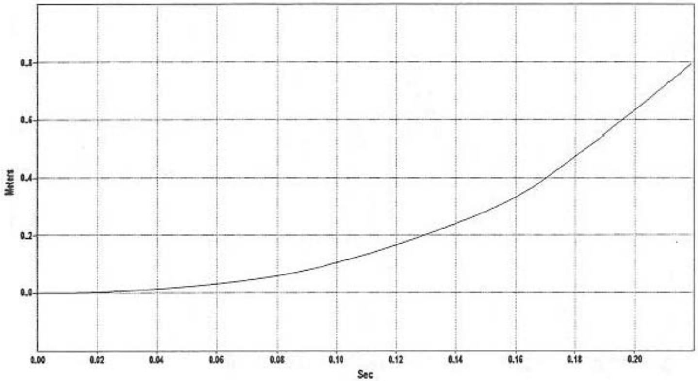
Figure C-33. Relative Longitudinal Occupant Displacement, Test BEST-11.
