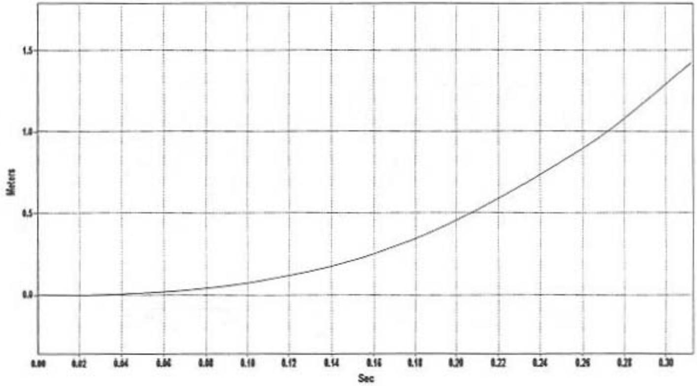
Figure C-3. Relative Longitudinal Occupant Displacement, Test BEST-3.
