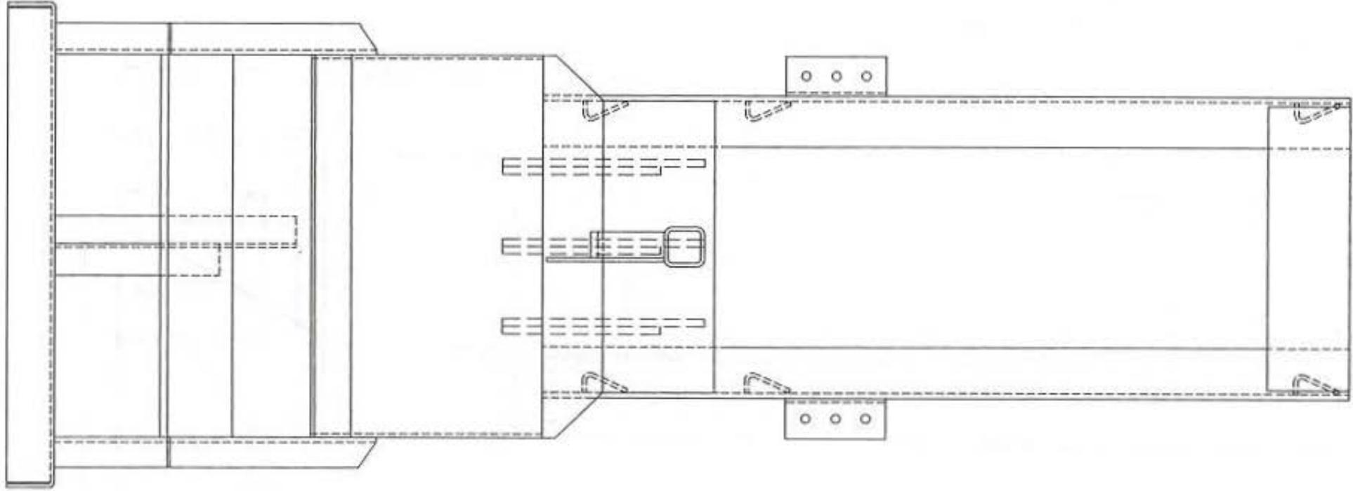
Figure 6. Side View of the BEST Impact Head for Tests BEST-8 through BEST-11.
