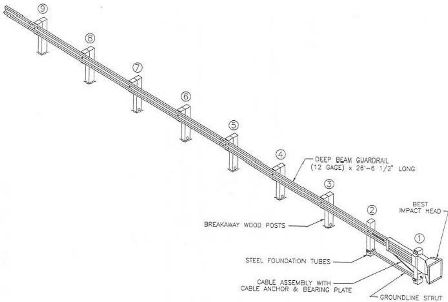
Figure 3. Schematic of the BEST system.
