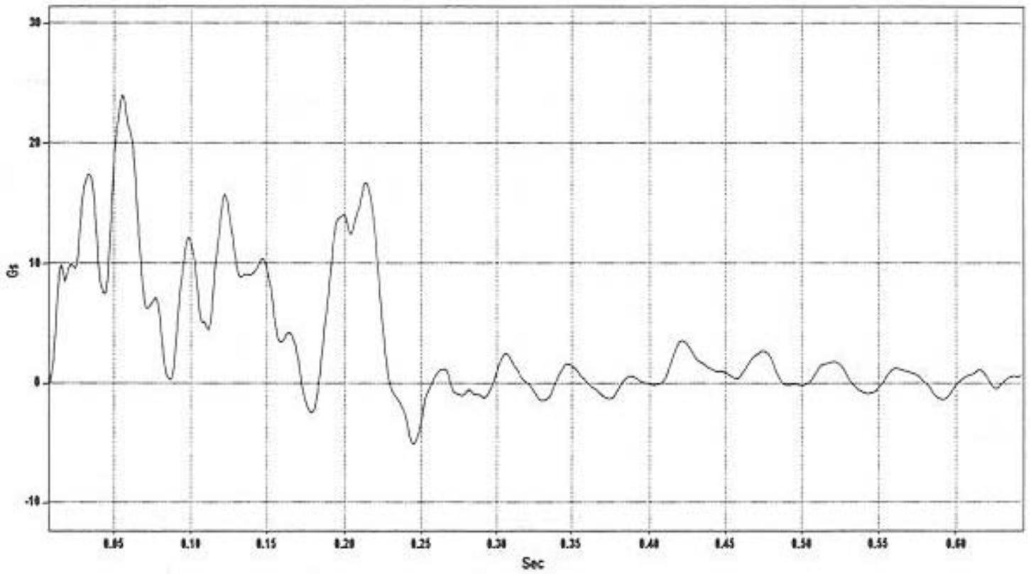
Figure C-13. Longitudinal Deceleration, Test BEST-8.
