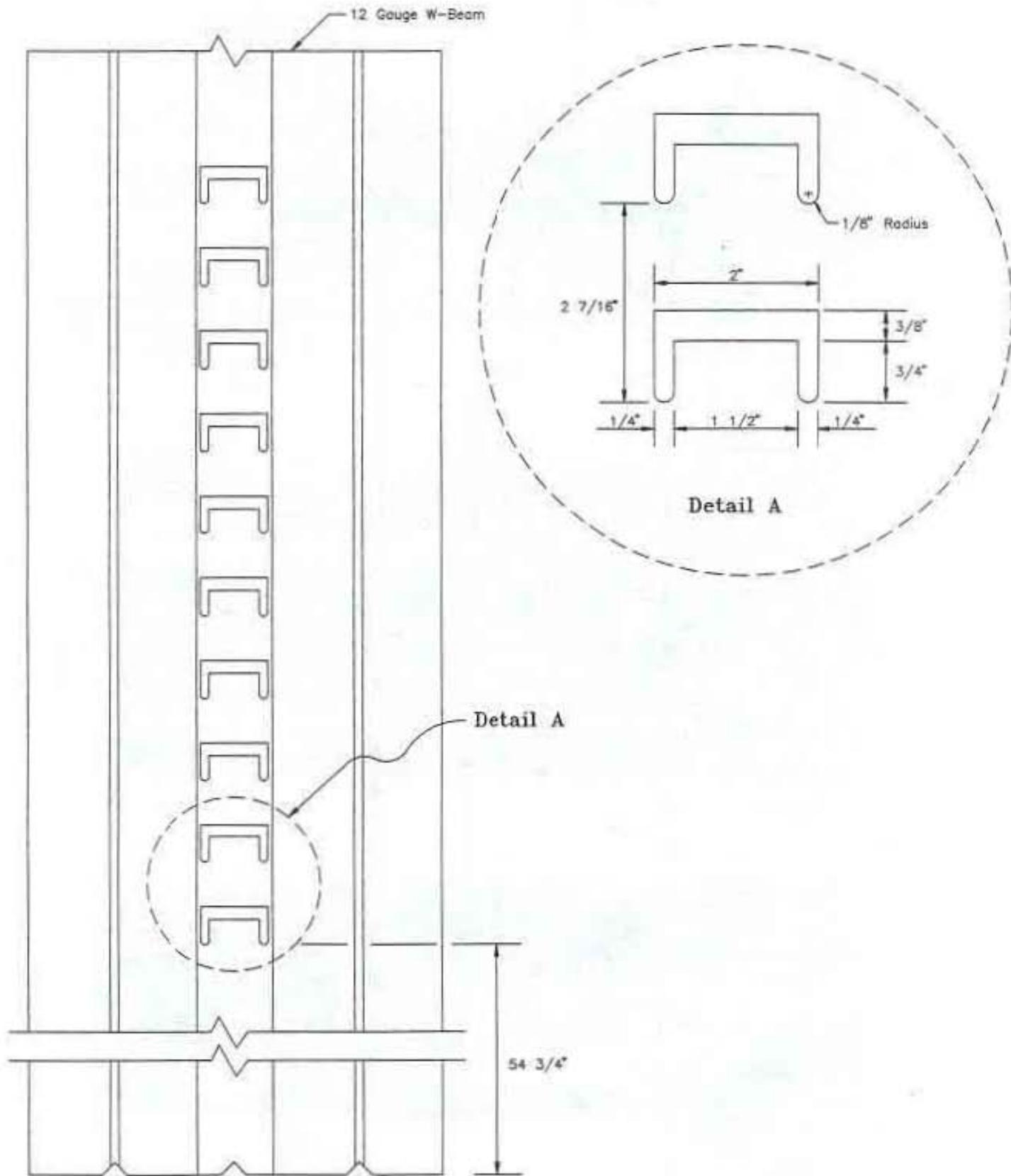
Figure 12. Breakaway Cable Anchor W-beam Attachment Details.
