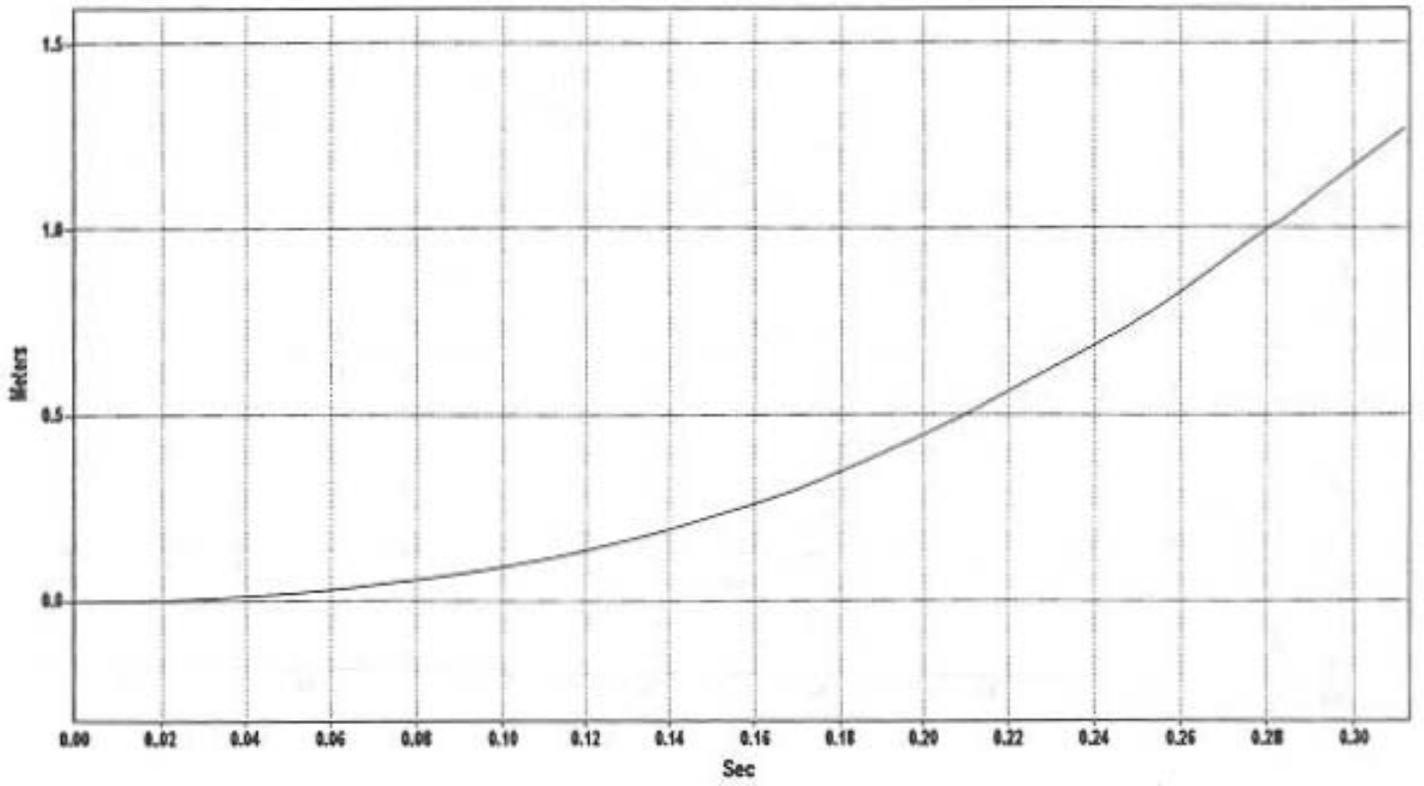
Figure C-6. Relative Lateral Occupant Displacement, Test BEST-3.
