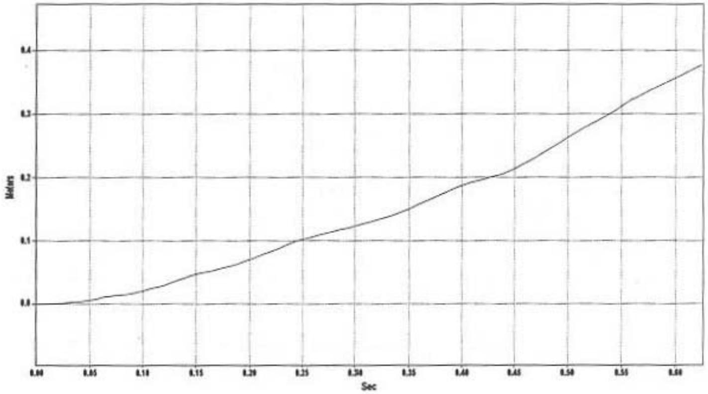
Figure C-24. Relative Lateral Occupant Displacement, Test BEST-9.
