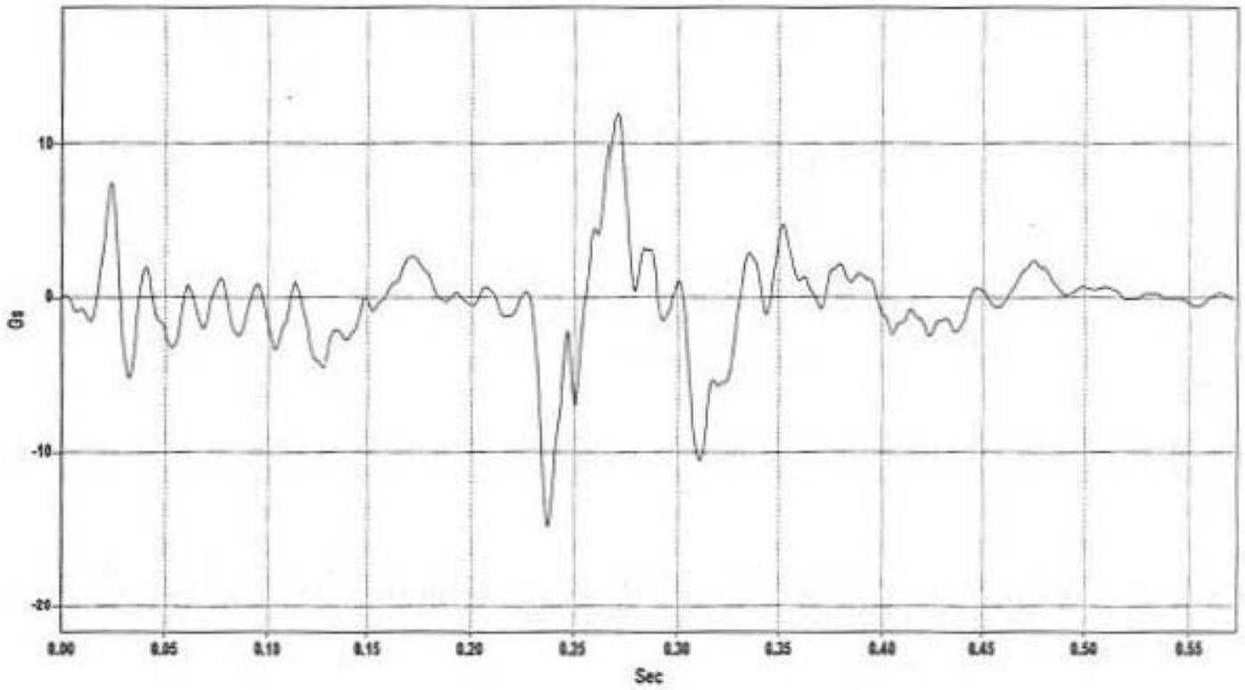
Figure C-28. Lateral Deceleration, Test BEST-10.
