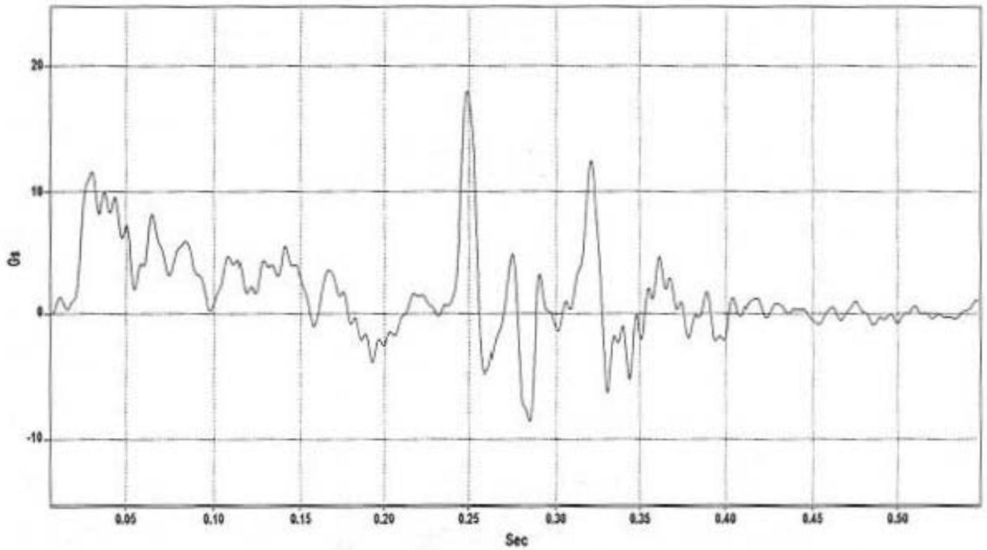
Figure C-25. Longitudinal Deceleration, Test BEST-10.
