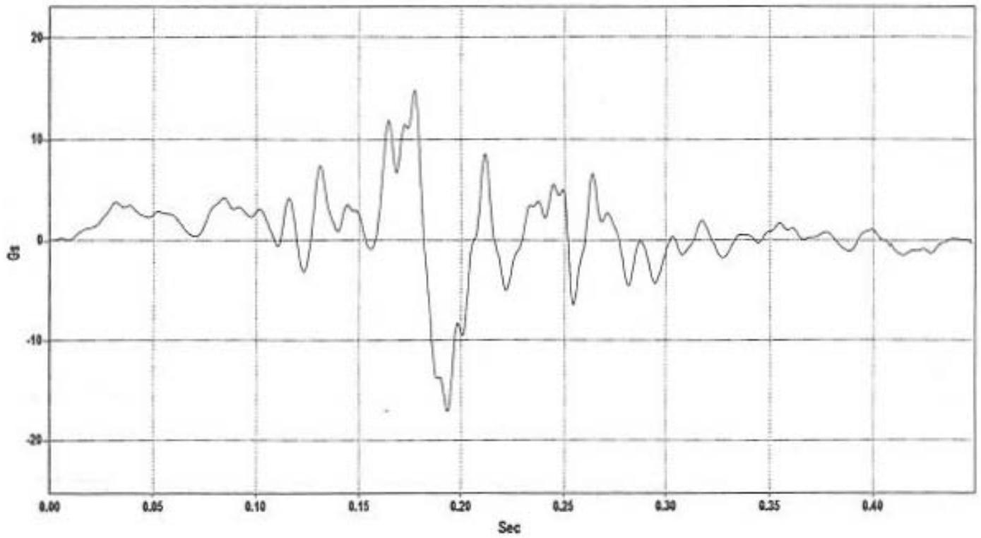
Figure C-34. Lateral Deceleration, Test BEST-11.
