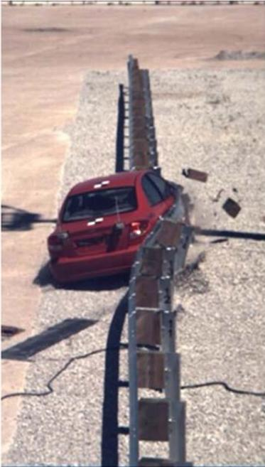
Figure 4. Test No. MGSMRH-1 Penetration
