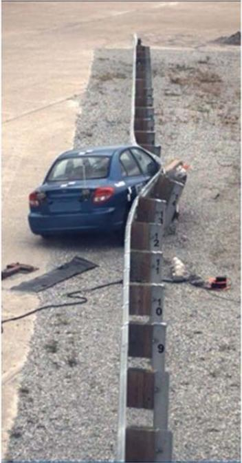
Figure 5. Test No. MGSMRH-2 Penetration
