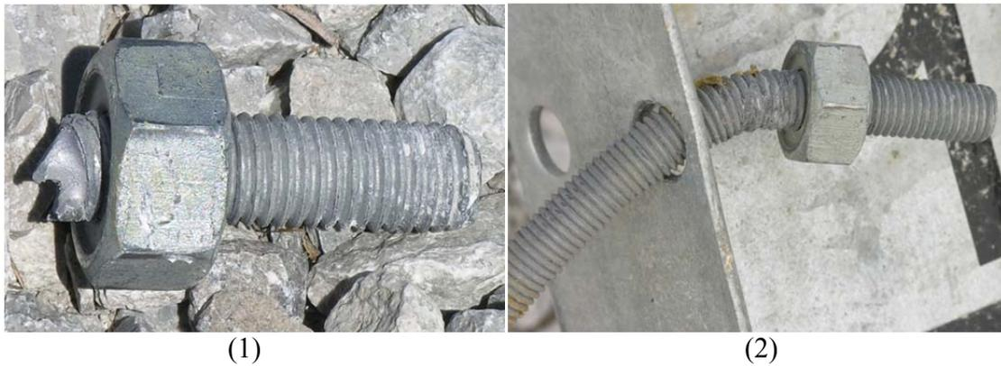
Figure 28. Blockout Bolt Failure Modes
