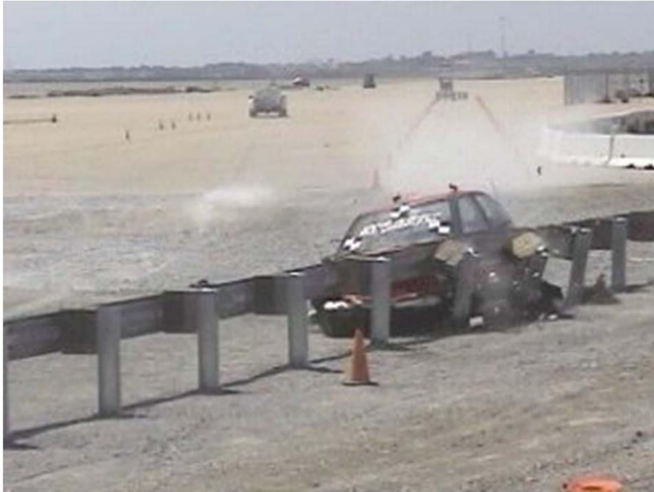
Figure 1. 820C Impact with MGS, test no. NPG-1
