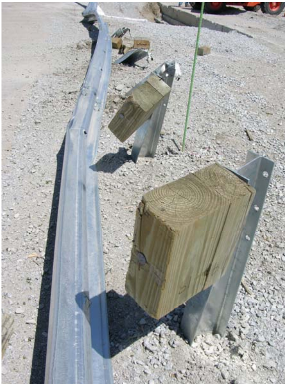
Figure 34. System Post Damage, Test No. LSC-1
