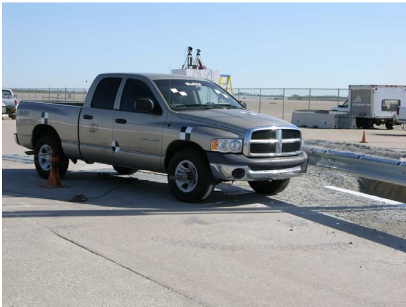
Figure 17. Test Vehicle, Test No. LSC-1
