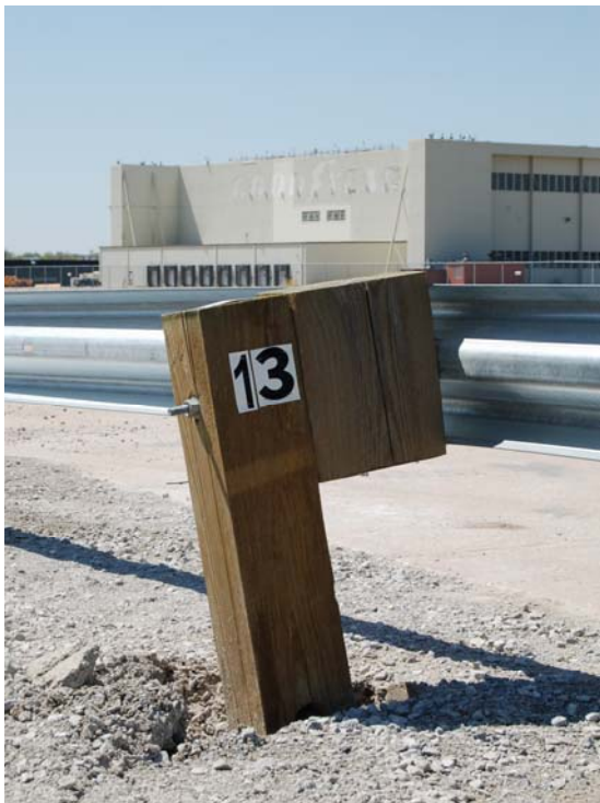
Figure 33. System Post Damage, Test No. LSC-1
