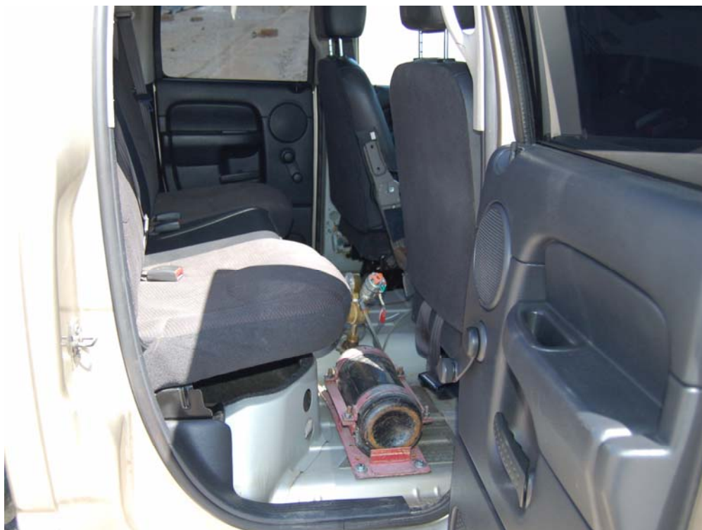
Figure 39. Occupant Compartment Deformation, Test No. LSC-1
