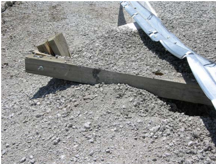
Figure 61. System Post Damage, Test No. LSC-2
