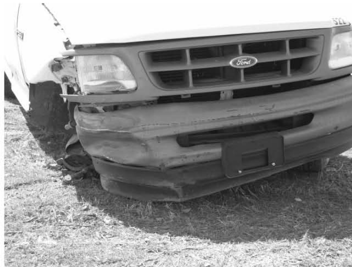
Figure 63. Vehicle Damage, Test SR-5
