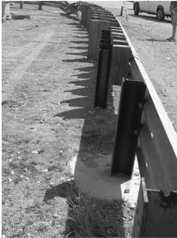
Figure 51. System Damage, Test SR-5
