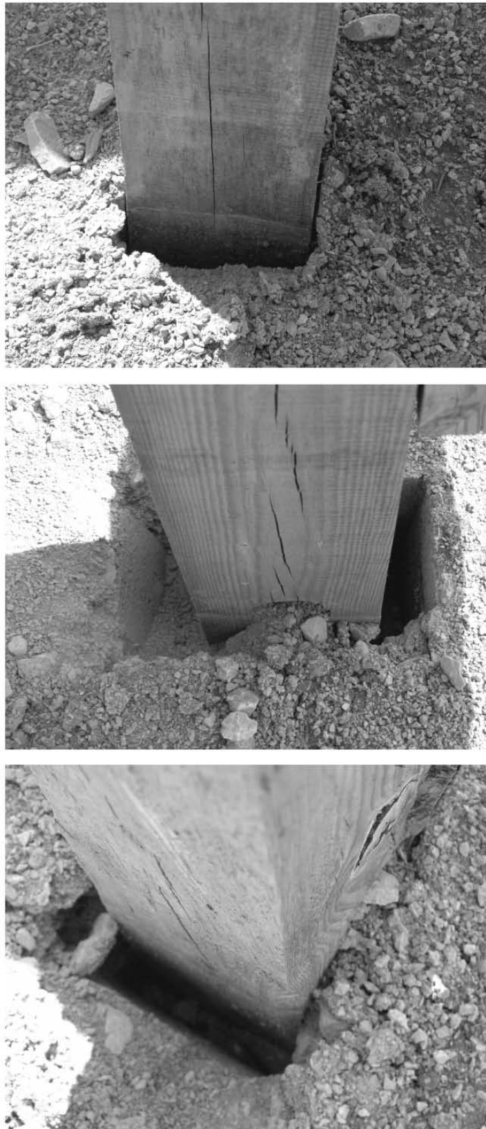
Figure 61. Soil Failure, Test SR-5
