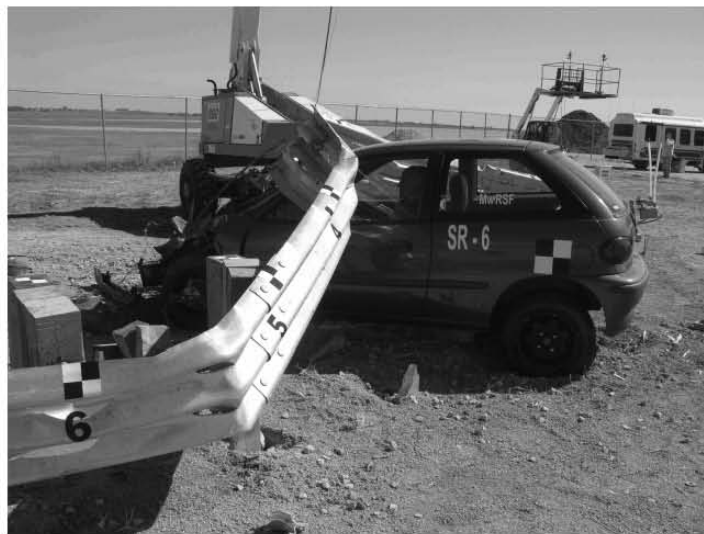
Figure 88. System Damage, Test SR-6
