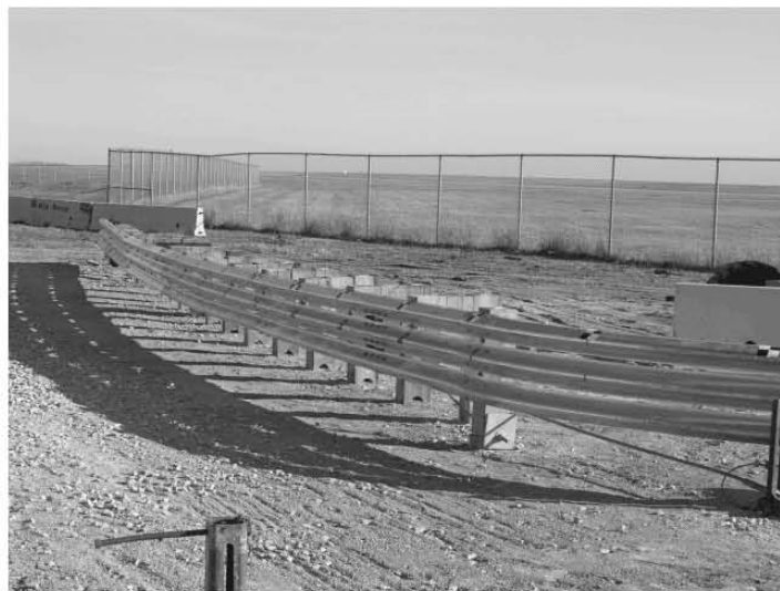
Figure 38. Short-Radius Nose Section Details
