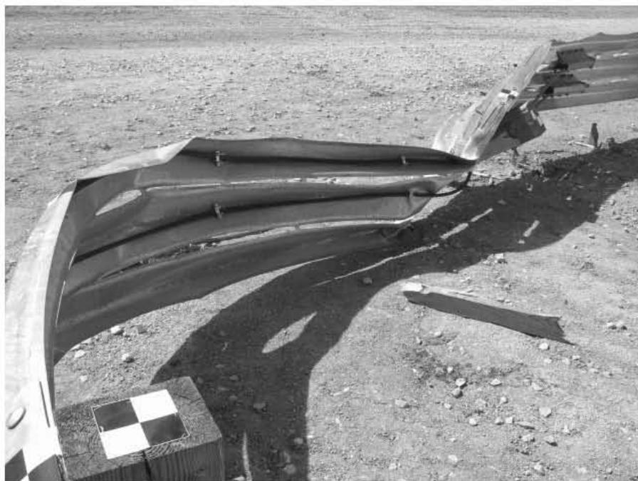
Figure 53. Damage to Nose Section, Test SR-5
