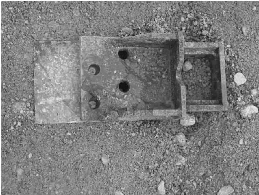
Figure 55. Cable Anchor Damage, Test SR-5
