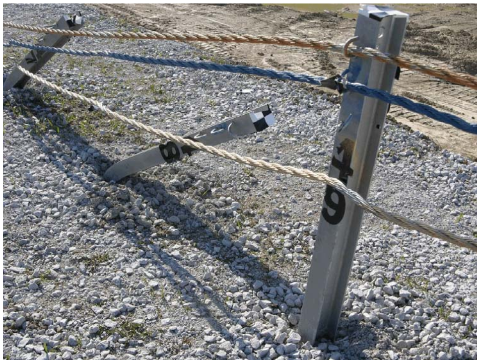
Figure 33. System Damage, Test CS-2
