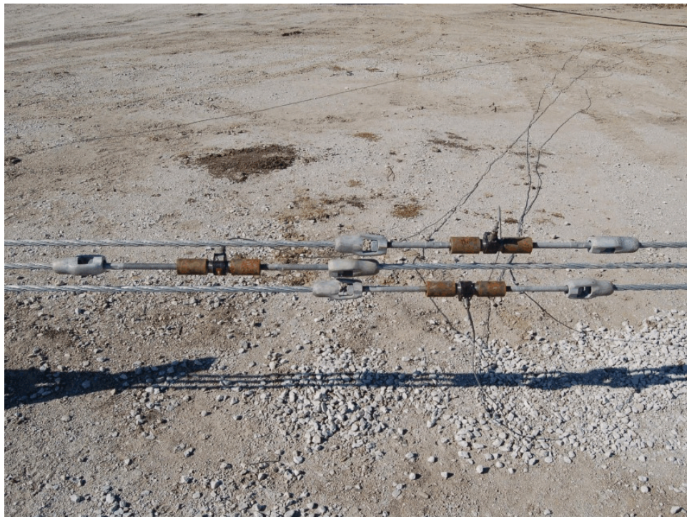
Figure 5. Upstream End Load Cell Positioning
