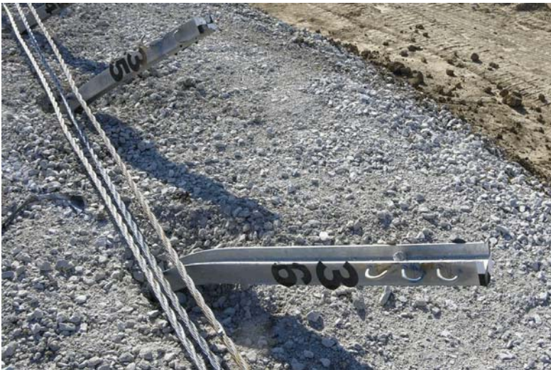
Figure 31. System Damage, Test CS-2
