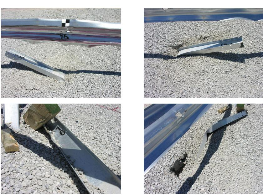
Figure 44. Post Nos. 15 and 16 Damage, Test No. MGSMRH-1
