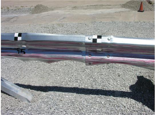
Figure 39. System Damage, Test No. MGSMRH-1
