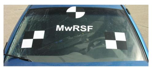
Figure 69. Vehicle Damage, Test No. MGSMRH-2
