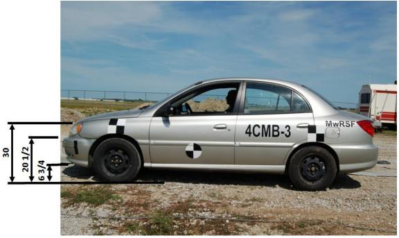
Figure 7. 1100C Front End Dimensions
