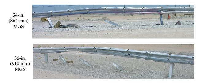
Figure 74. System Damage Comparison
