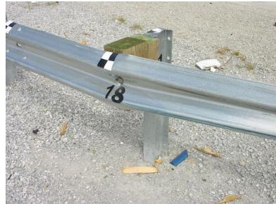
Figure 67. Post Damage, Test No. MGSMRH-2
