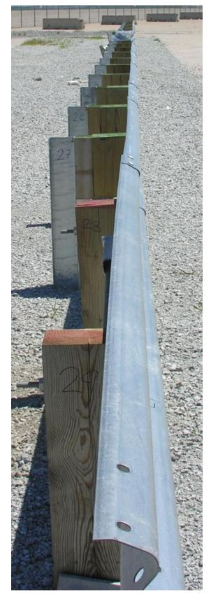
Figure 37. System Damage, Test No. MGSMRH-1
