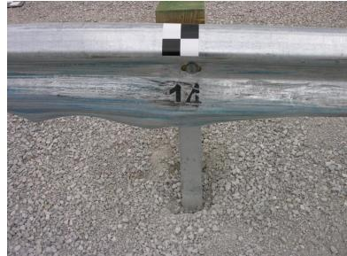
Figure 65. Post Damage, Test No. MGSMRH-2
