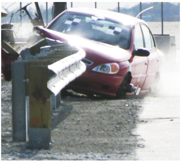
Figure 5. Test No. 2214MG-3, Rail Snags Under the Hood
