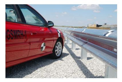
Figure 34. Impact Location, Test No. MGSMRH-1
