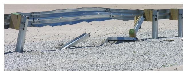
Figure 38. System Damage, Test No. MGSMRH-1
