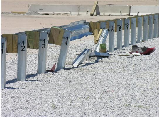
Figure 36. System Damage, Test No. MGSMRH-1
