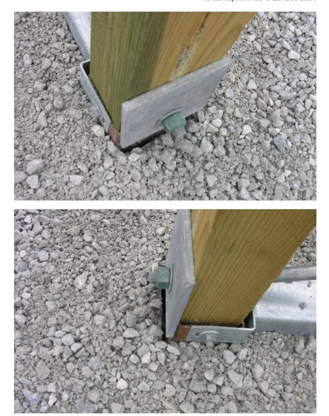
Figure 63. Soil Gap at Upstream End Anchor, Test No. MGSMRH-2
