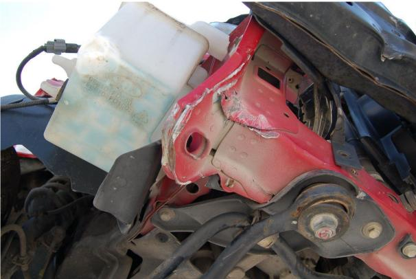
Figure 49. Undercarriage Damage, Test No. MGSMRH-1
