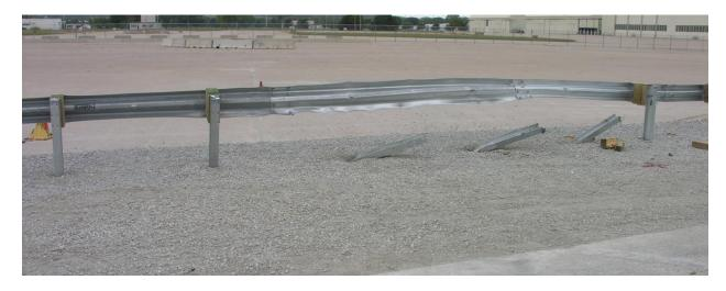
Figure 62. System Damage, Test No. MGSMRH-2
