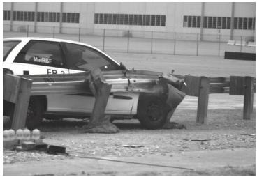
Figure 1. Test No. FR-3, Potential for Wheel Snag
