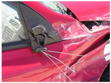
Figure 47. Vehicle Damage, Test No. MGSMRH-1
