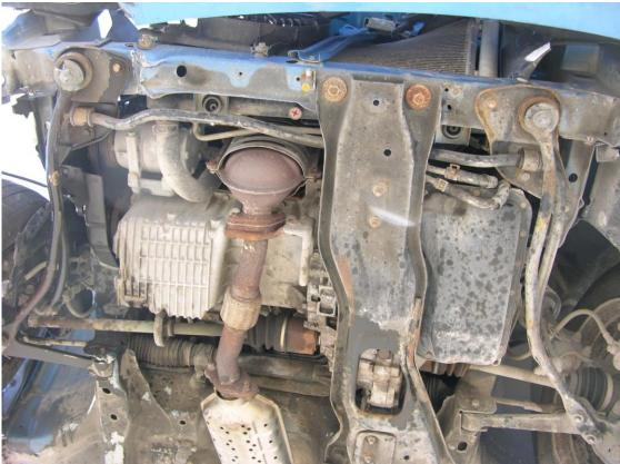
Figure 71. Undercarriage Damage, Test No. MGSMRH-2
