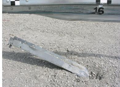
Figure 66. Post Damage, Test No. MGSMRH-2
