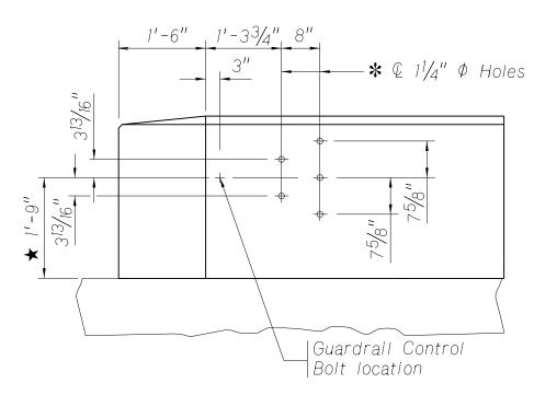
\*As an alternate method, the contractor shall furnish and cast into the concrete an approved welded assembly consisting of threaded inserts, held accurately to the template of the holes shown. Inserts are to be complete with galvanized plate washers and galvanized \%\text{8}"\Phi x 2" cap screws. The insert assembly shall be a standard product of a reputable manufacturer of such items and be capable of resisting a shear load of 80,000 lbs.
