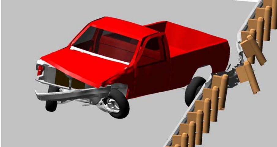
Figure 54. Vehicle Pocketing during Impact of Wood Post System in Rigid Mow Strip.
