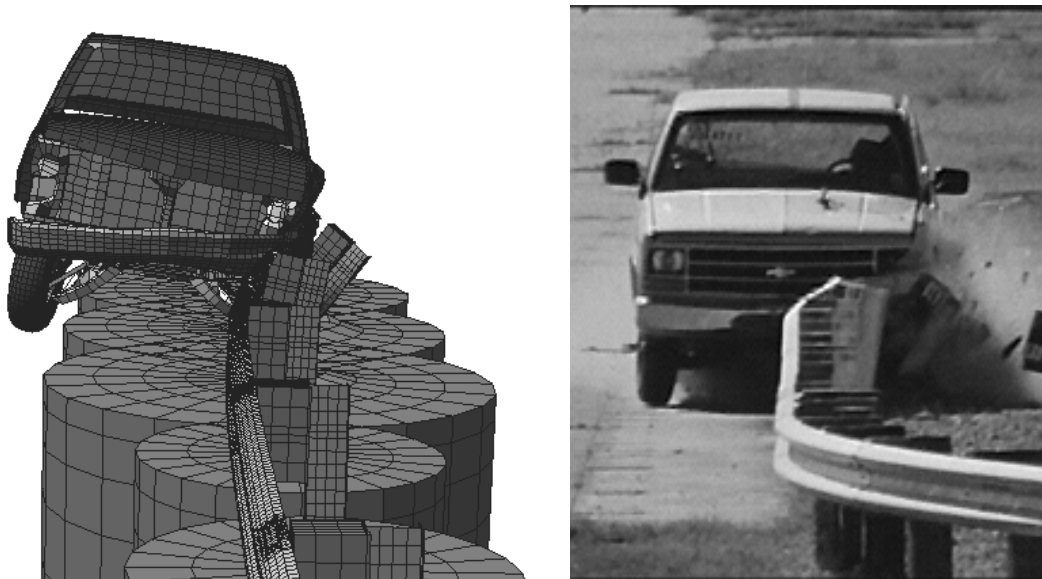
Figure 46. Side-by-Side Comparison of Numerical Simulation and Crash Test.
