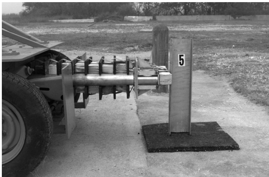
Figure 12. Asphalt Mow Strip Bogie Test with Rubber Mat.
