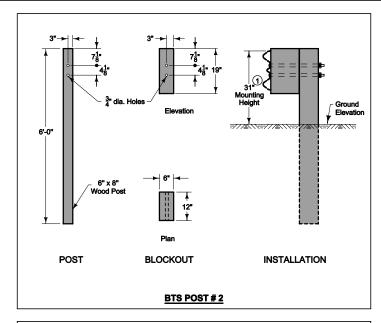
Guardrail mounting height at barrier connection is 32 inches. Transition guardrail mounting height down to 31 inches over the length of the Barrier Transition Section.
