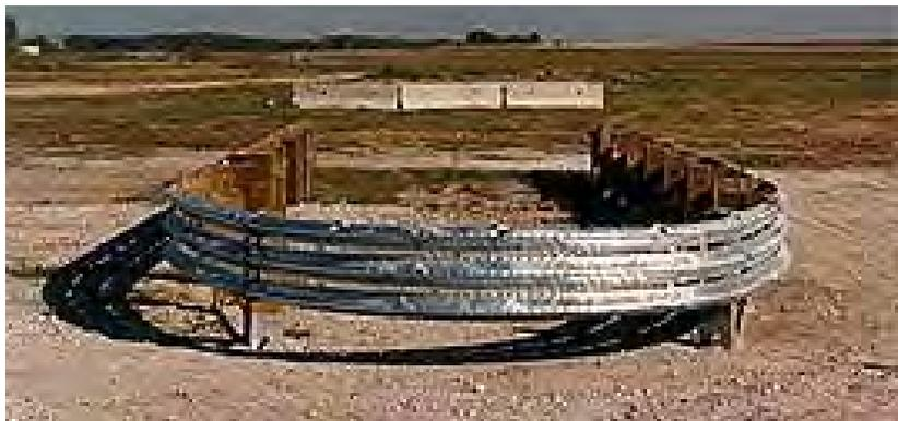
**Figure 31. Bullnose Attenuator.**
