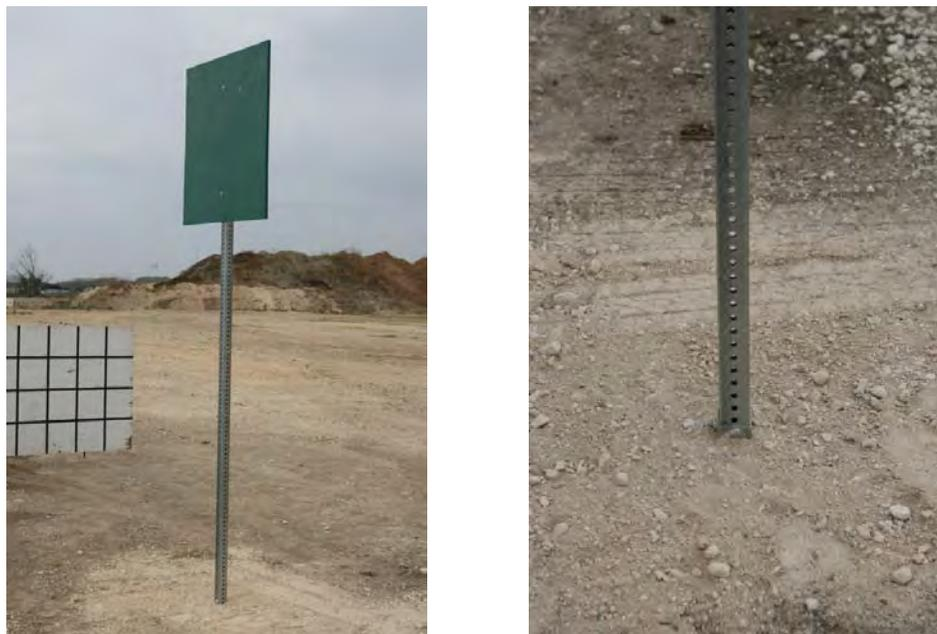
**Figure 67. Perforated Square Steel Tubing Sign Support prior to Testing.**
