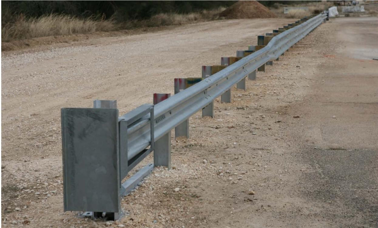
**Figure 83. G9 Thrie Beam Guardrail prior to Testing.**
