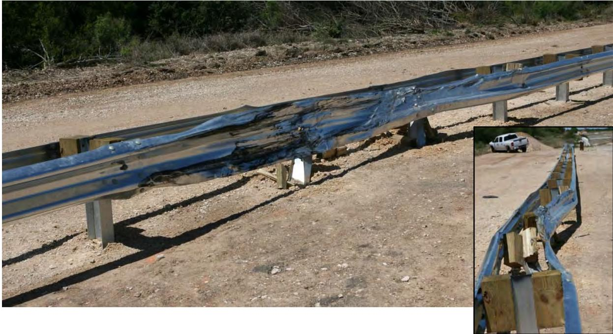
**Figure 56. G4(1S) W-Beam Median Barrier after *MASH* Test 3-11.**
