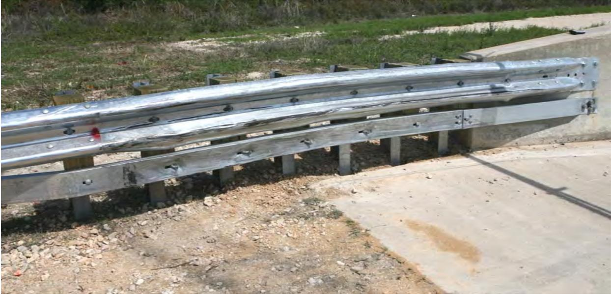
**Figure 61. PennDOT W-Beam Transition after *MASH* Test 3-21.**
