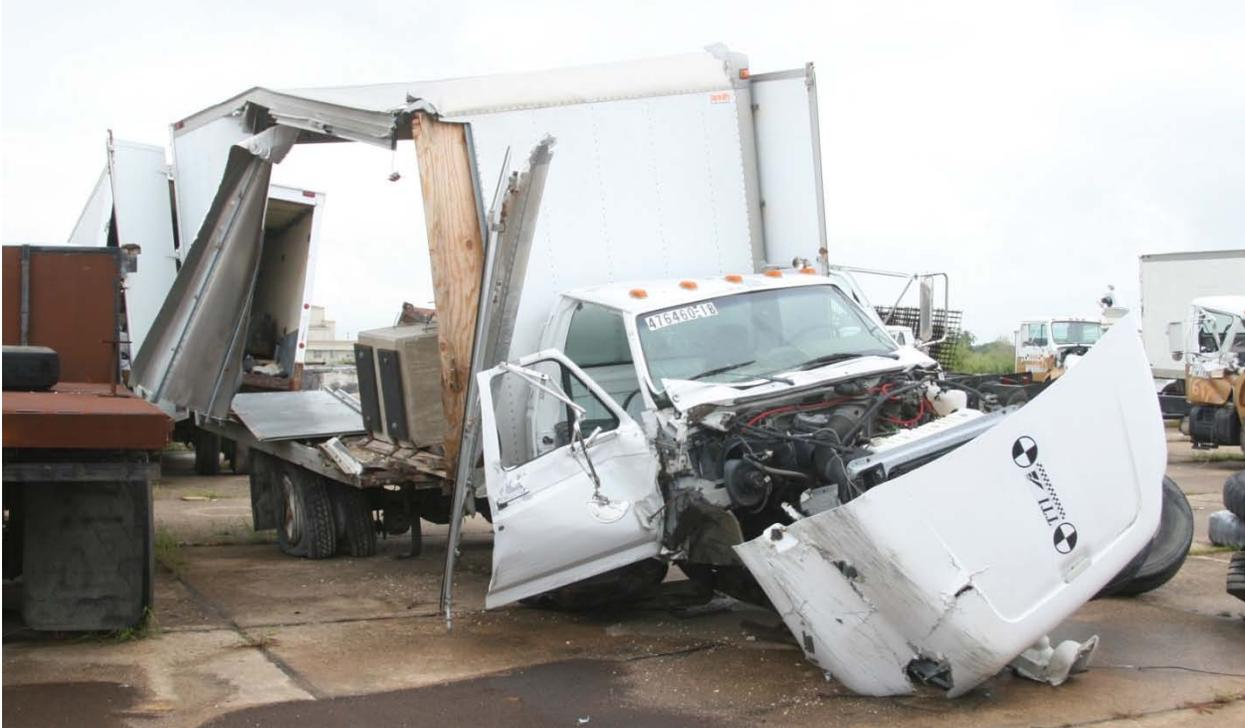
**Figure 41. Test Vehicle after *MASH* test 4-12 on the 32-inch New Jersey Safety Shape Barrier.**
