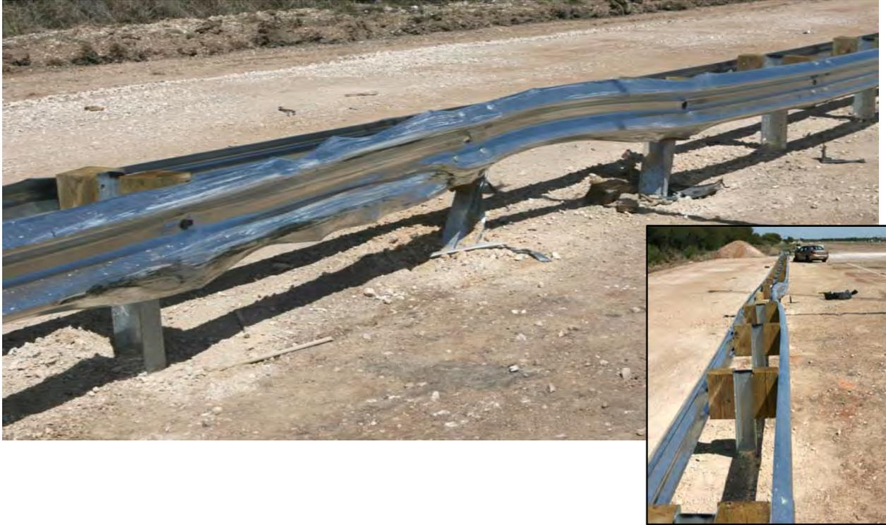
**Figure 53. G4(1S) W-Beam Median Barrier after *MASH* Test 3-10.**
