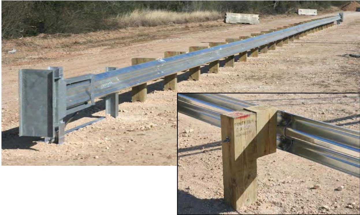
**Figure 47. G4(2W) W-Beam Guardrail Prior to Testing.**
