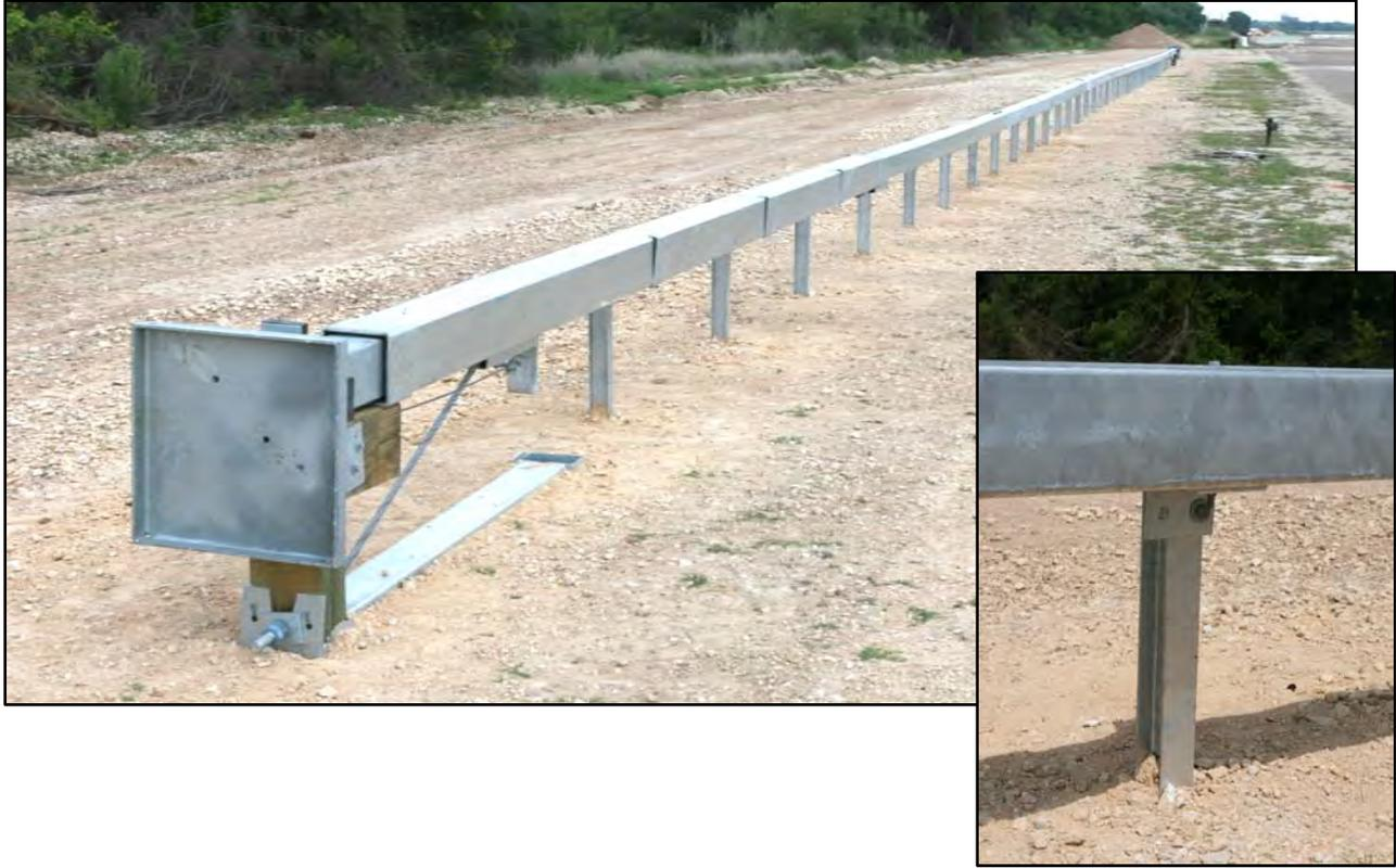
**Figure 73. G3 Weak Post Box-Beam Guardrail prior to Testing.**
