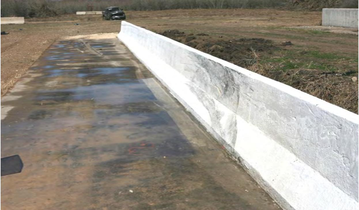
**Figure 43. 32-inch New Jersey Shape Barrier after *MASH* Test 3-11.**
