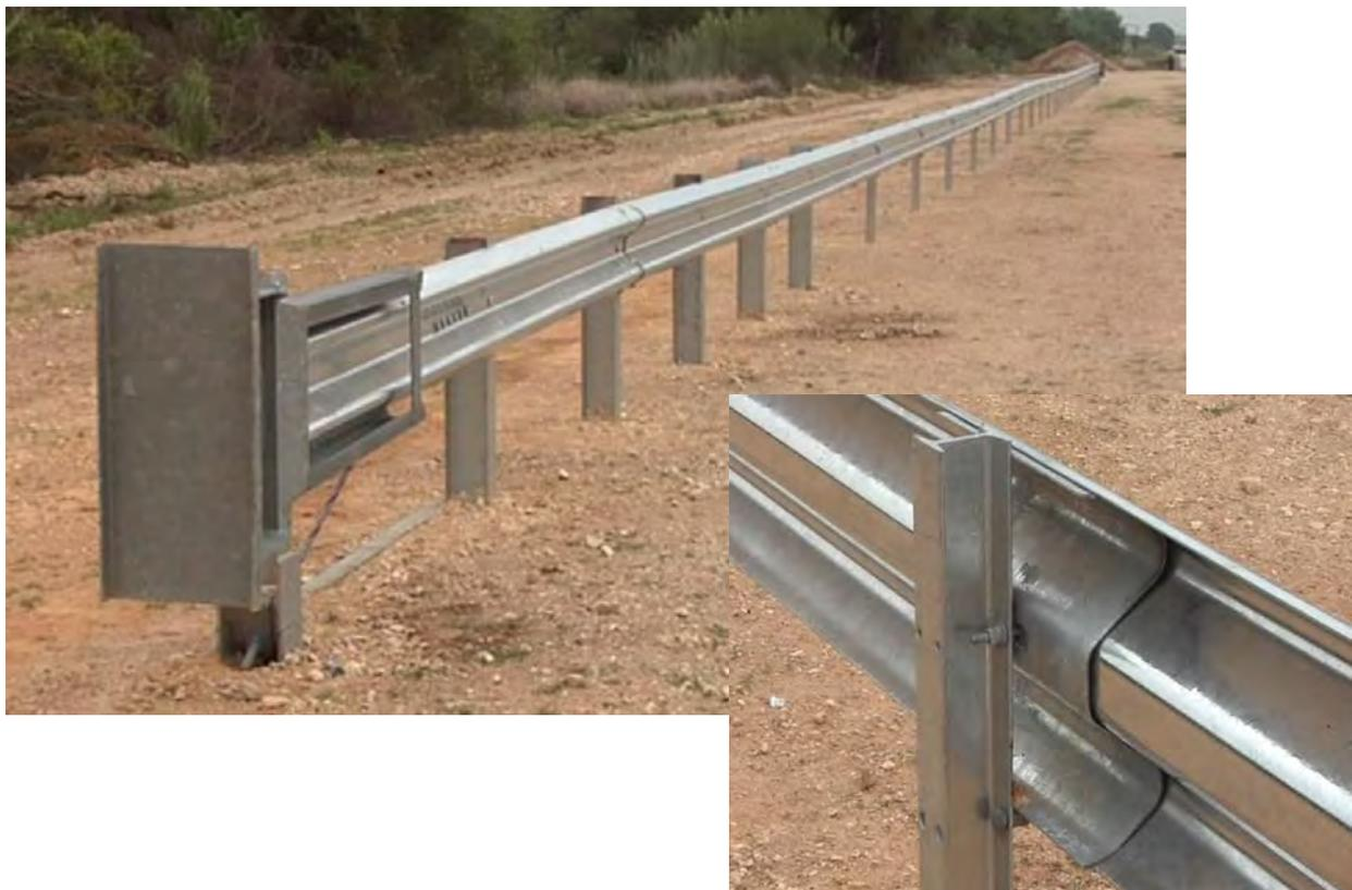
**Figure 78. Modified G2 Weak Post W-Beam Guardrail prior to Testing.**
