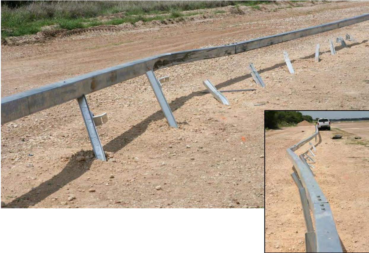
**Figure 74. G3 Weak Post Box-Beam Guardrail after *MASH* Test 3-11.**
