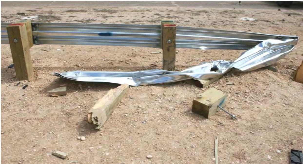
**Figure 48. G4(2W) W-Beam Guardrail after MASH Test 3-11.**
