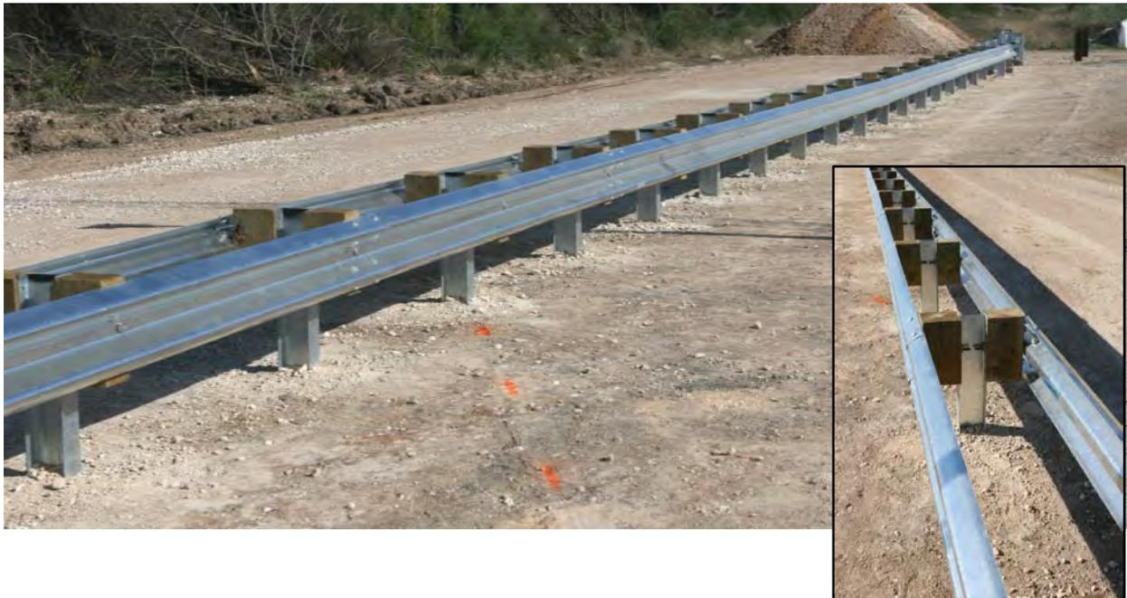
**Figure 52. G4(1S) W-Beam Median Barrier Prior to Testing.**
