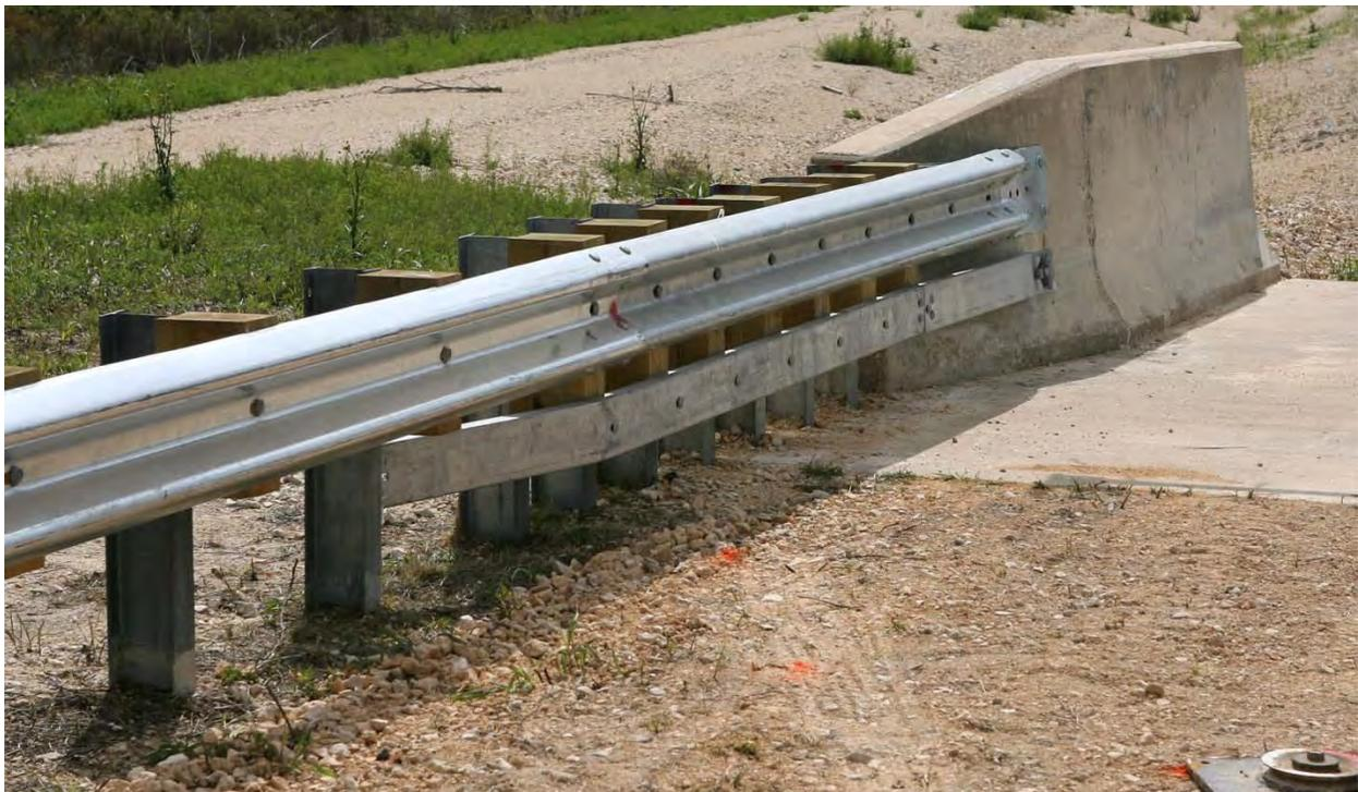
**Figure 60. W-Beam Transition prior to Testing.**
