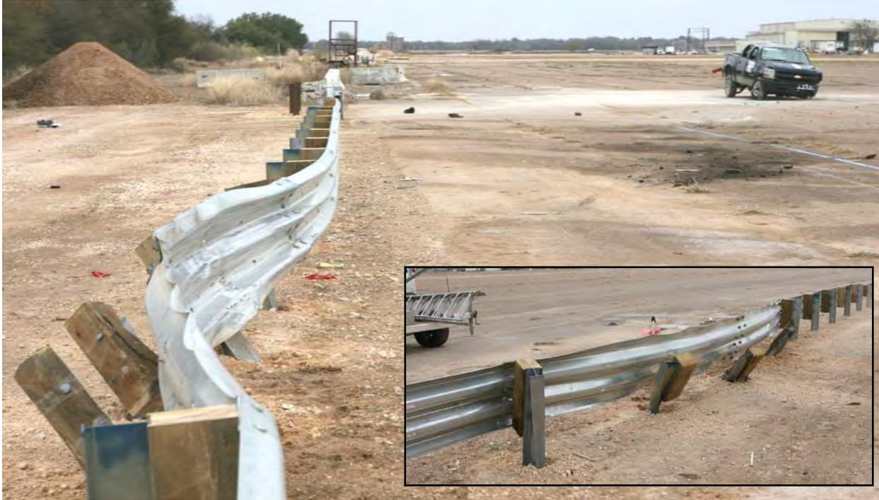
**Figure 84. G9 Thrie Beam Guardrail after *MASH* Test 3-11.**
