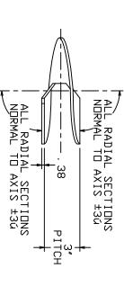
HELIX MUST BE FORMED BY MATCHING METAL DIE (SIDE VIEW OF TRUE HELICAL FORM)
