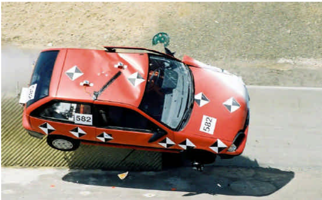
Figure 2-12 Test vehicle 582 during the Test (the vehicle rolled over twice to the left after landing)
