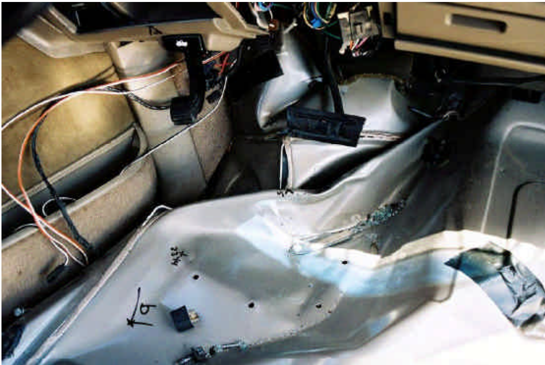
Figure 2-24 Vehicle floorboard deformation after Test 583
