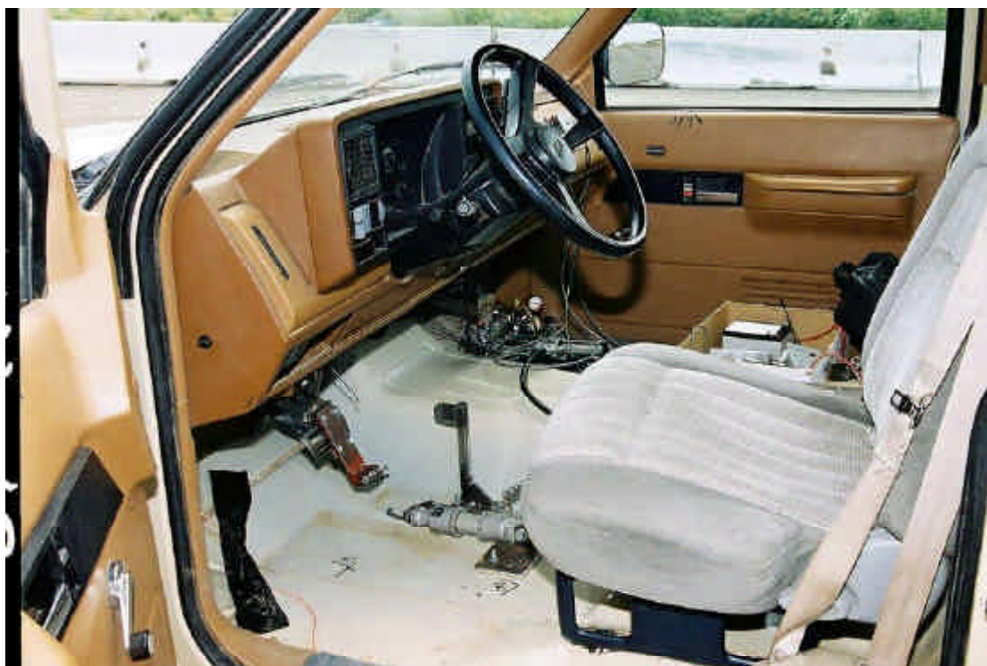
Figure 2-38 Interior and floorboard of test vehicle prior to Test 585
