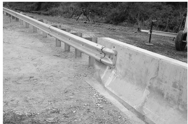
FIGURE 1 Transition system before crash test.
