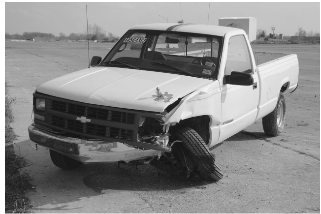
FIGURE 3 Damage to vehicle after crash test.
