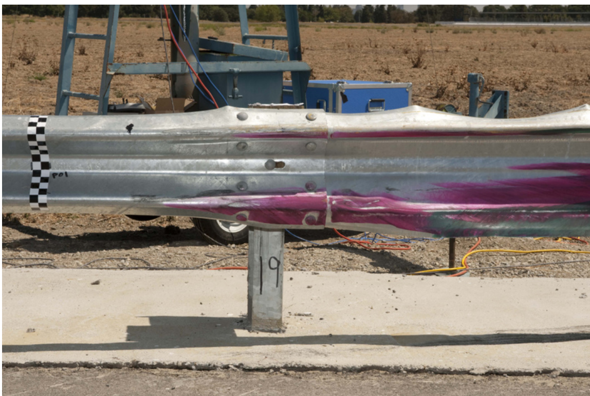
Figure 2-39 – Impact Point after Test 659
