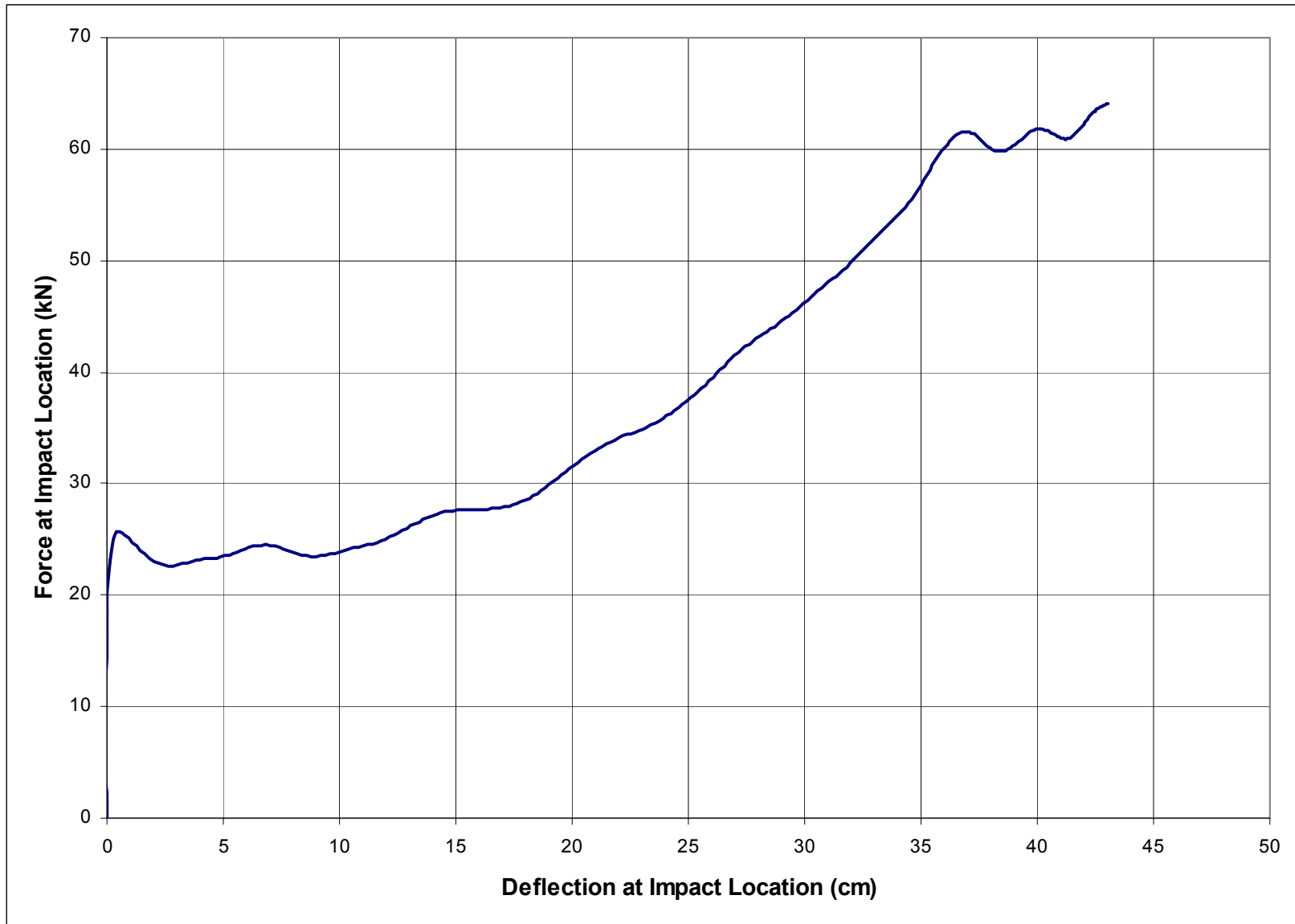
Figure C-6. Force-Deflection Plot Derived from Strain Gauge Data, Test MPR-3
