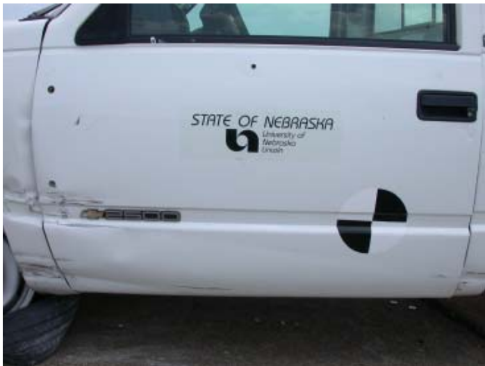
Figure 52. Vehicle's Left-Side Damage, Test PR-1
