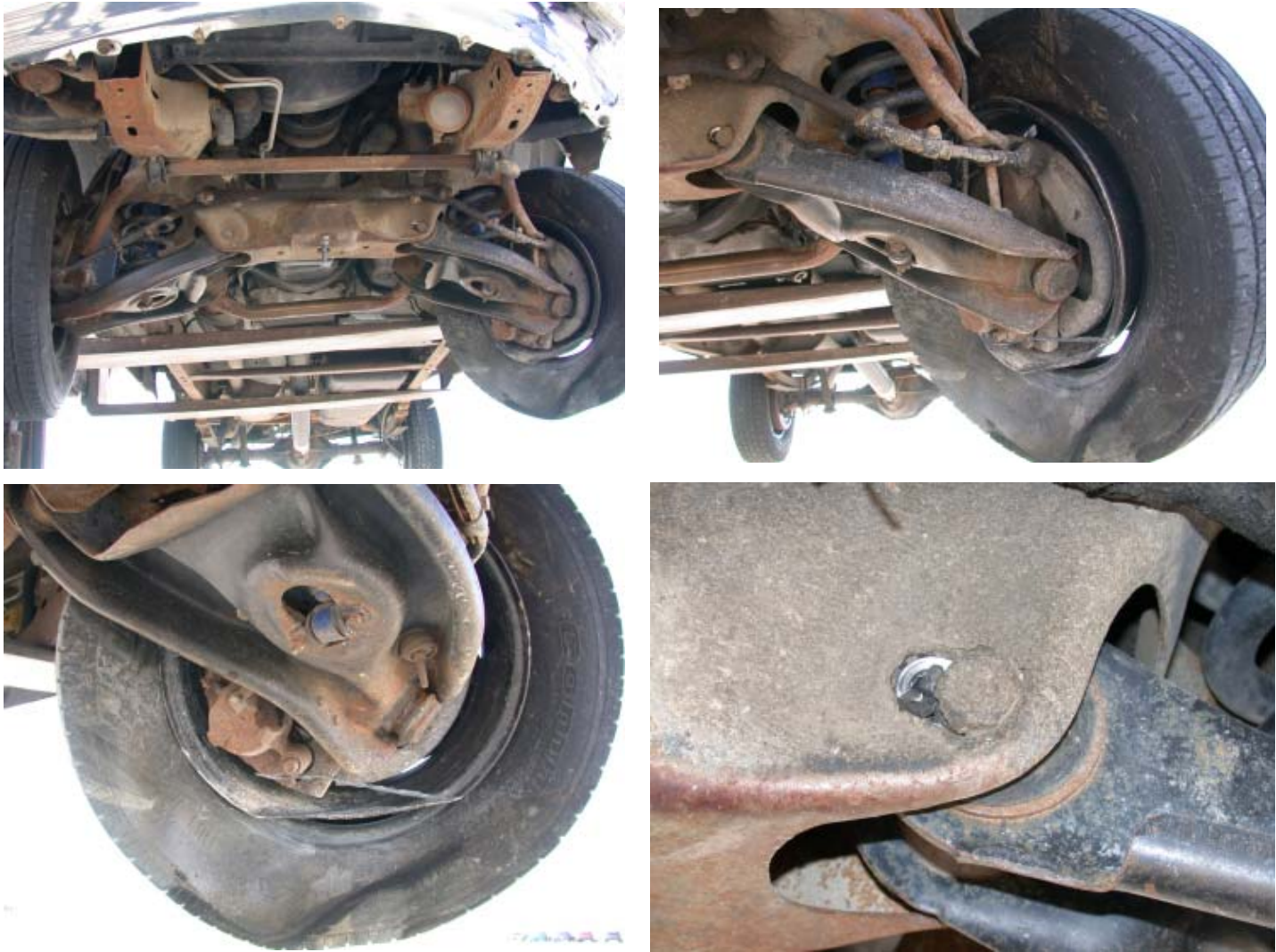
Figure 53. Vehicle Undercarriage Damage, Test PR-1
