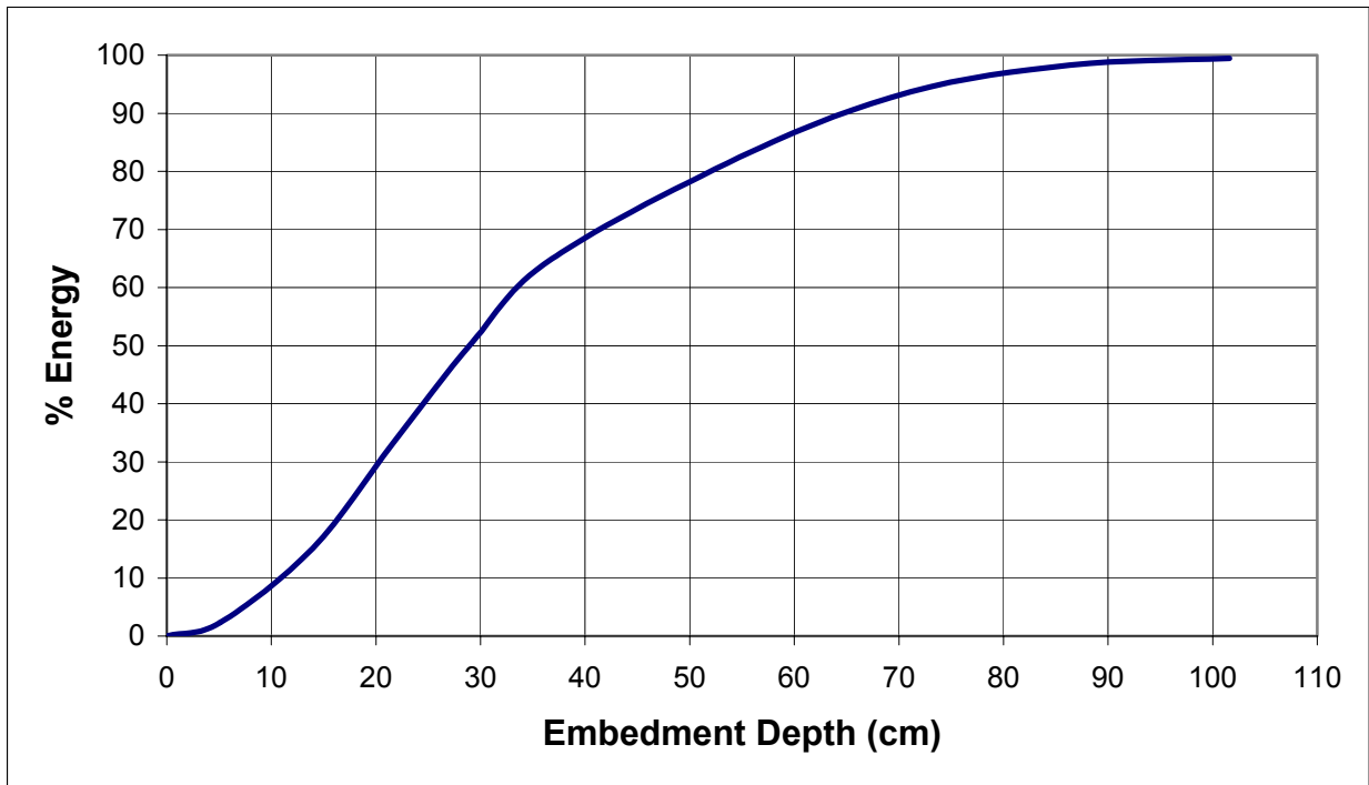
Figure 63. Percentage of Absorbed Energy versus Embedment Depth in Soil, Test SSF-9
