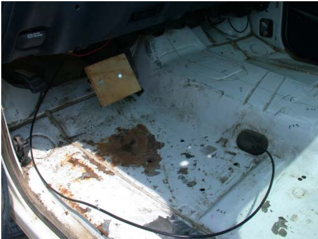
Figure 54. Occupant Compartment Deformations, Test PR-1
