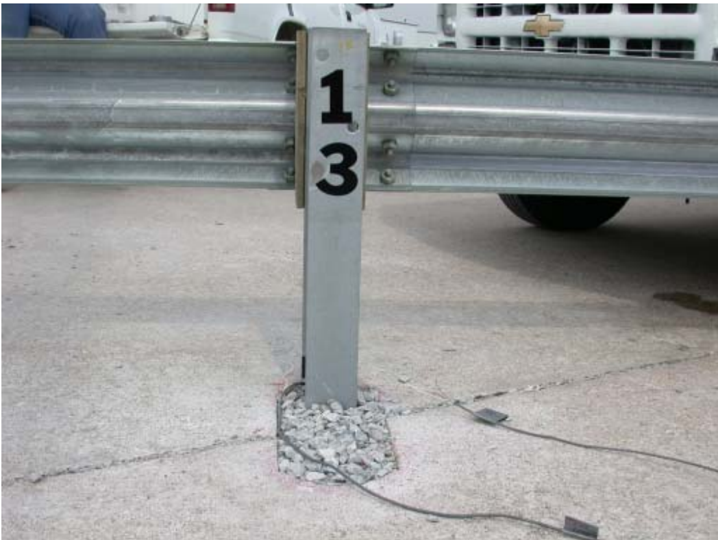
Figure 34. Typical Post Installed in Elongated Drilled Hole
