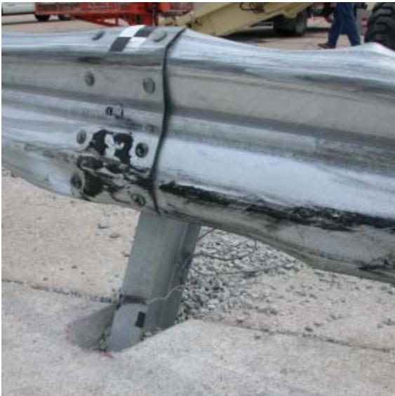
Figure 48. Post Nos. 12 and 13 Damage, Test PR-1
