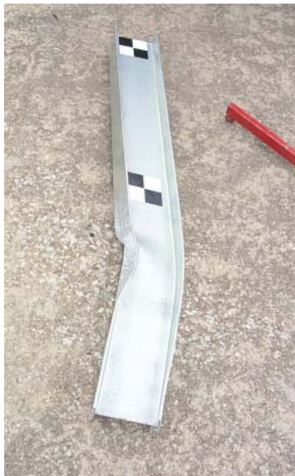
Figure 17. Post Damage, Bogie Test MPR-7
