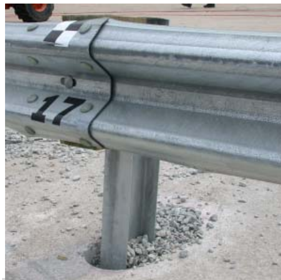
Figure 50. Post Nos. 16 and 17 Damage, Test PR-1
