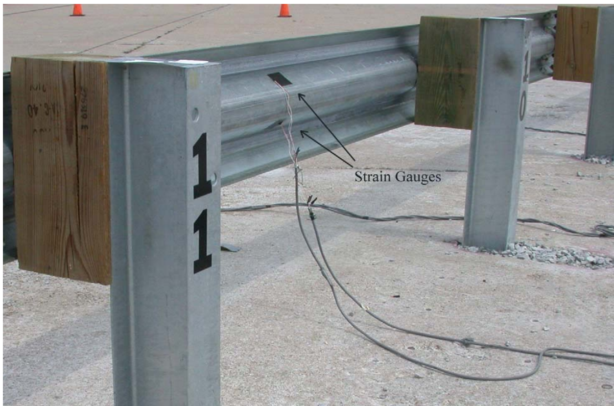
Figure 27. Location of Strain Gauges on Guardrail
