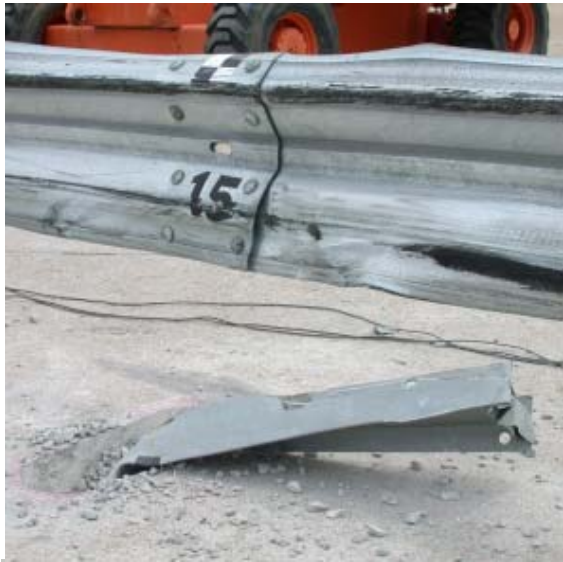
Figure 49. Post Nos. 14 and 15 Damage, Test PR-1
