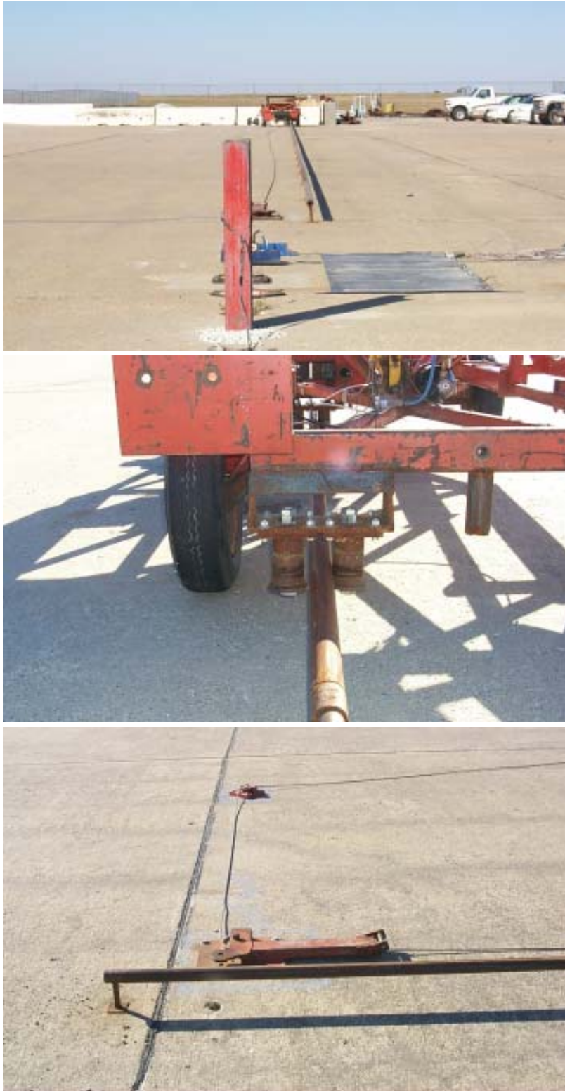
Figure 14. Bogie Tow and Guidance
