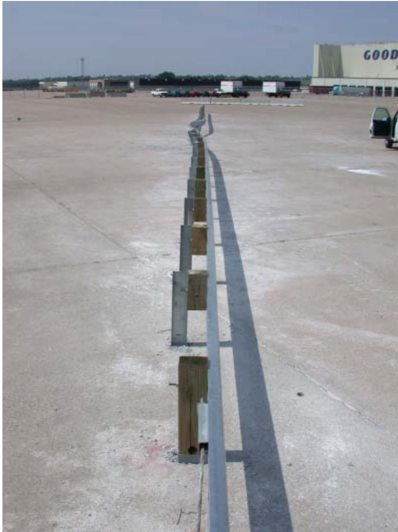
Figure 45. W-beam Guardrail System Damage, Test PR-1
