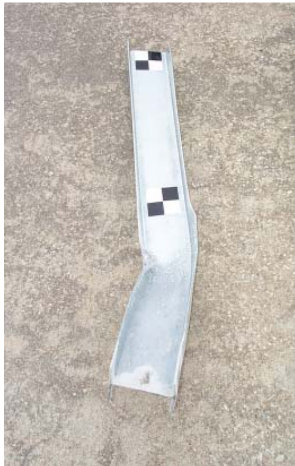
Figure 18. Post Damage, Bogie Test MPR-8
