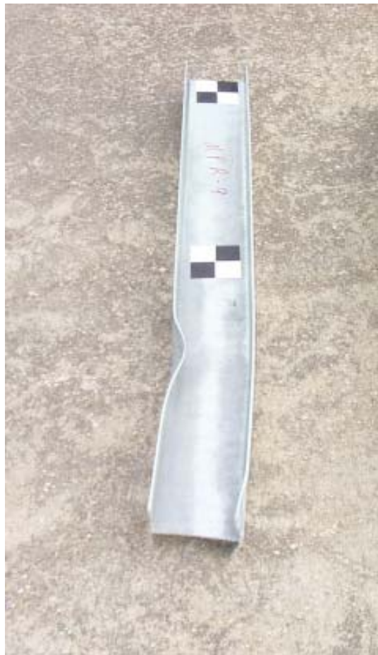
Figure 19. Post Damage, Bogie Test MPR-9
