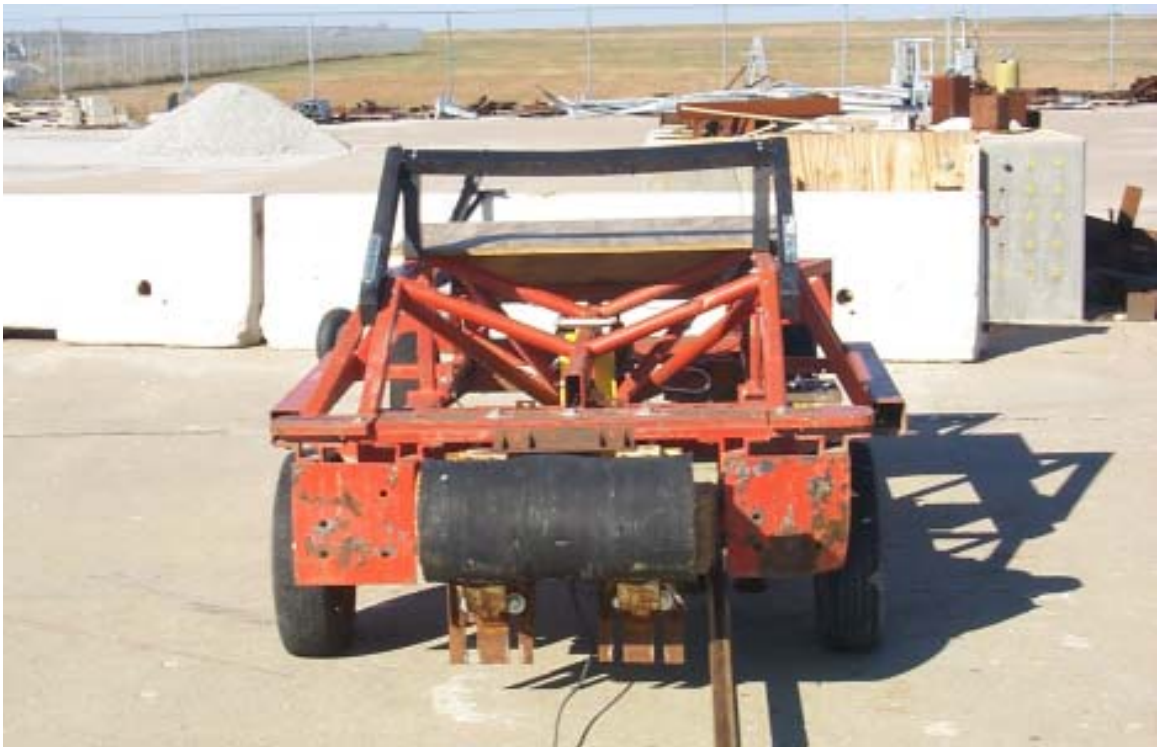
Figure 13. Rigid Bogie Vehicle
