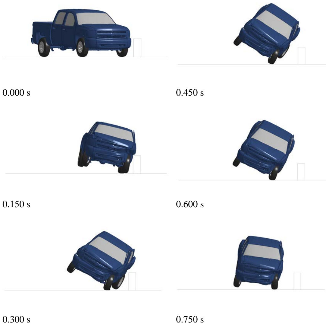
Figure 3.5 Sequential Photographs of FE Simulation with 29-inch Barrier Height.
