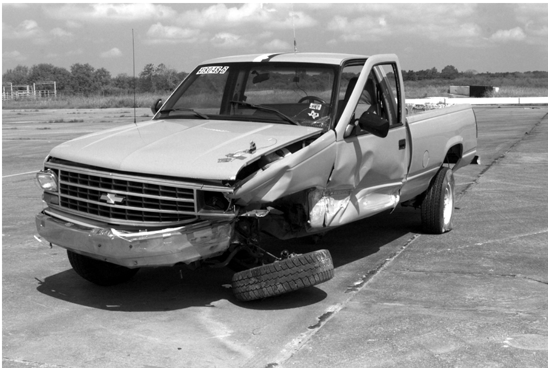
Figure 3.15 NCHRP Report 350 2000P Suspension after NCHRP Report 350 TL-3 Crash Test (15) .
