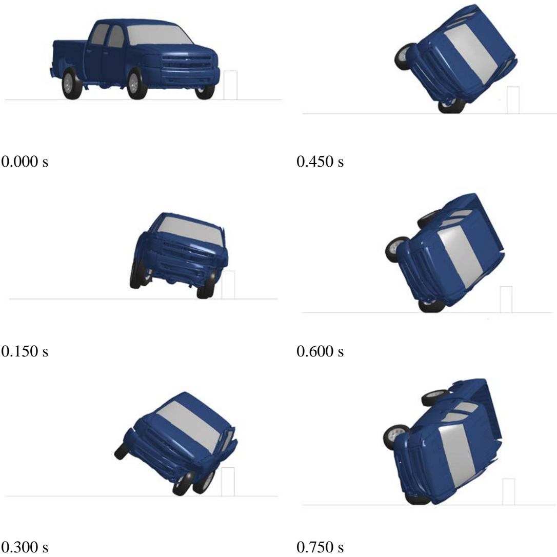
Figure 3.3 Sequential Photographs of FE Simulation with 27-inch Barrier Height.
