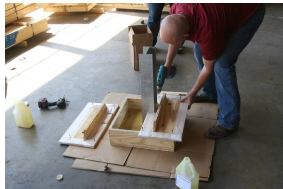
Figure 7: Installing top plates on mold after placement of foam mixture.
