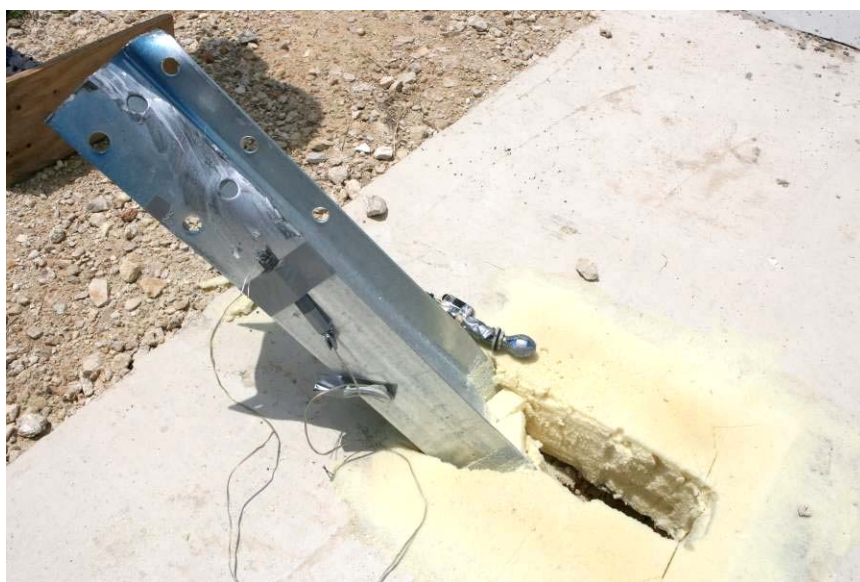
Figure 21: Post in two part urethane foam after test B2.
