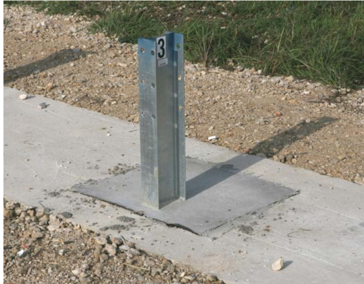
Figure 22: Post in full-strength unreinforced concrete wedge prior to test B3.
