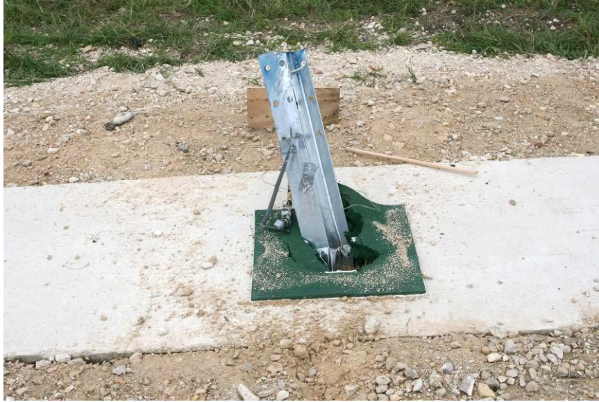
Figure 25: Post with TopHat™ recycled rubber mat after test B4.
